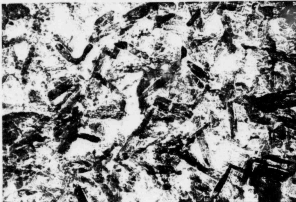
FIGURE 4--TEM micrograph of the rutile form of \text{TiO}_2 . 200000 X.
