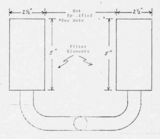
NOTE: Use available "els" and "T's" to assemble the filters such that the unit will fit into the 5 gal. container (  $10^{1}_{2}$ " dia.)
