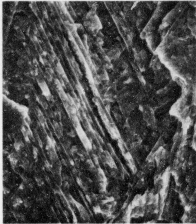
Figure 14. Hydrogen induced intermittent brittle crack propagation in a grain of TiCode-12 with hydrogen concentration above 5000 ppm. Note secondary interface cracking in the center.
