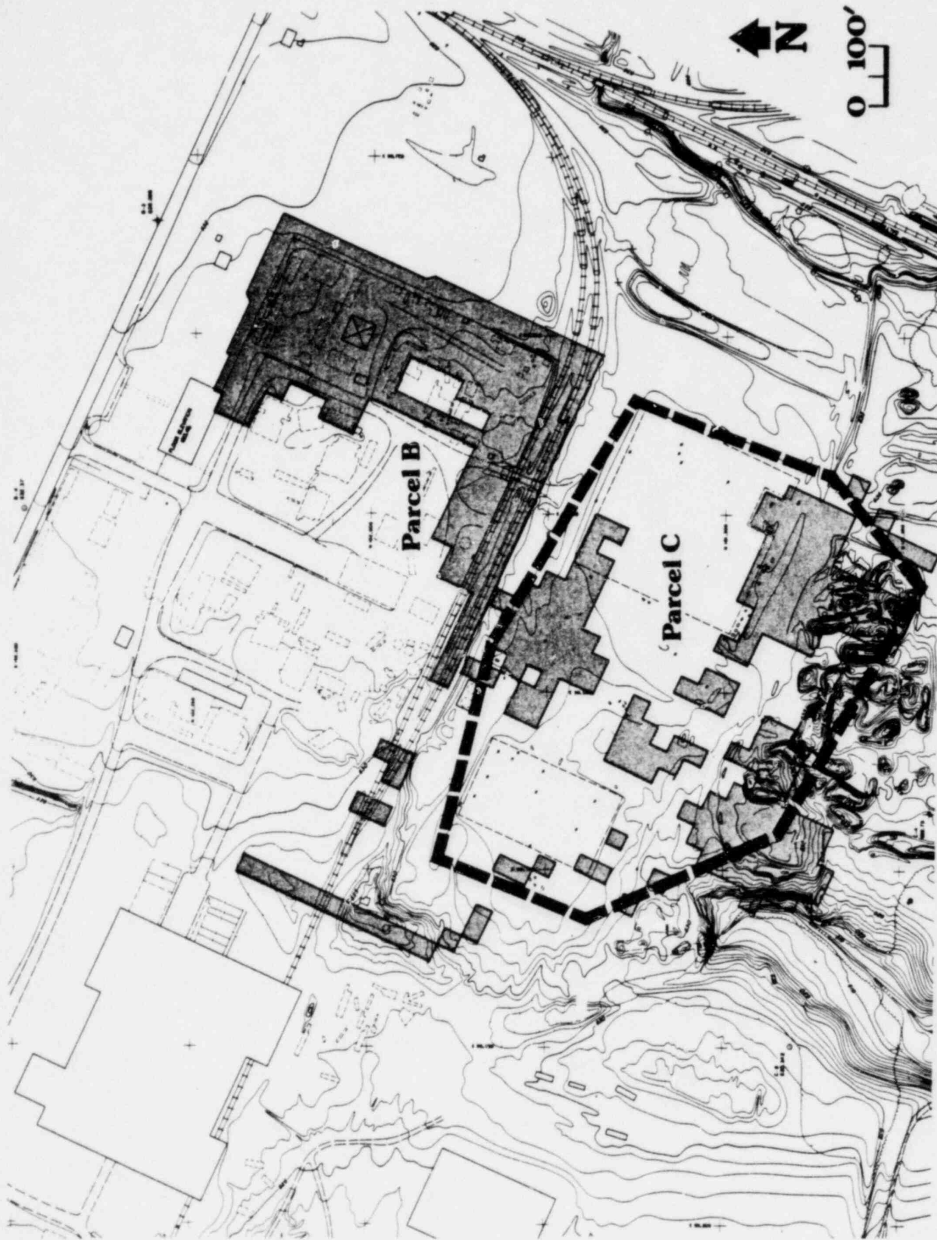
Figure 6. Location of Radioactively Enriched Soil, Greater than Background, and Outline of Control Area
