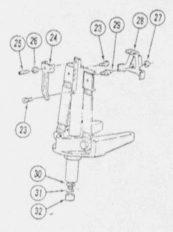
23 - Screw, Mounting 24 - Bracket, Pt. No. NO141FN 25 - Screw 25 - Nut. Locking
