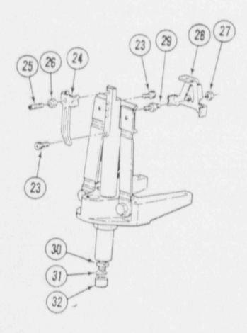
23 - Screw, Mounting 24 - Bracket, Pt. No. NO141FN 25 - Screw 26 - Nut, Locking
