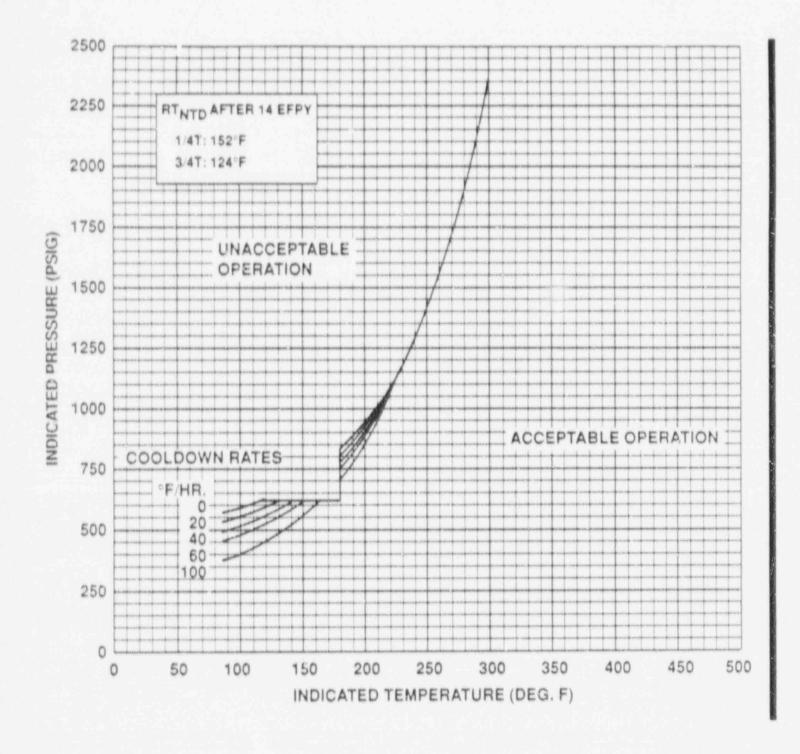
Figure 3.4-3 Farley Unit 2 Reactor Cooling System Cooldown Limitations Applicable for the First 14 EFPY.
