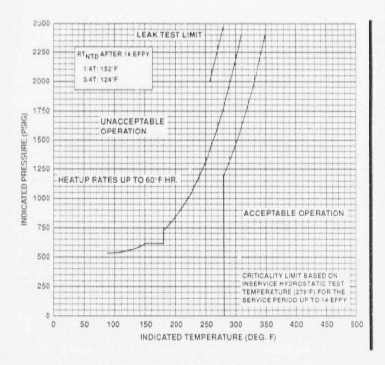
Figure 3.4-2 Farley Unit 2 Reactor Coolant System Heatup Limitations Applicable for the First 14 EFPY.
