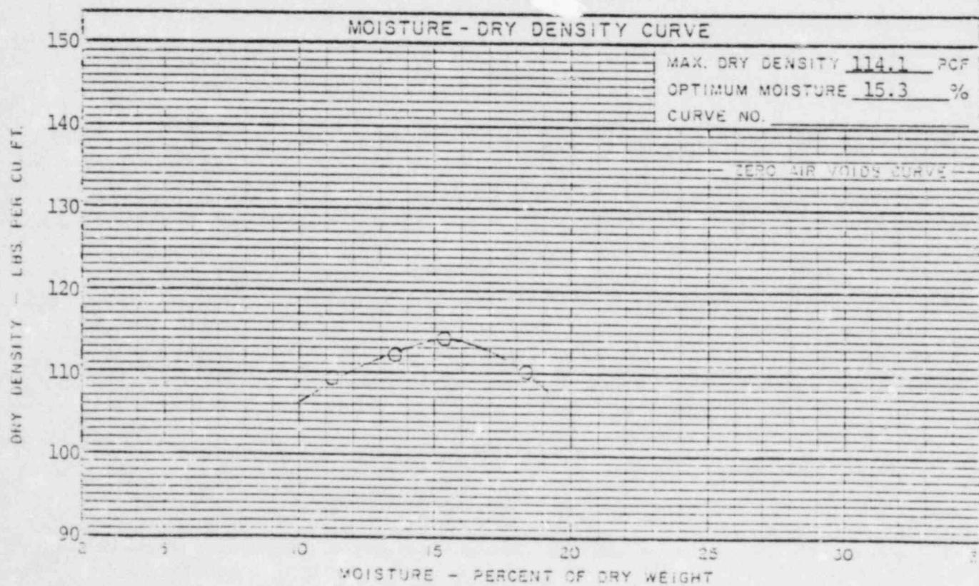
COMPACTION TEST PROCEDURE ASTM-D-698-78 METHOD A
