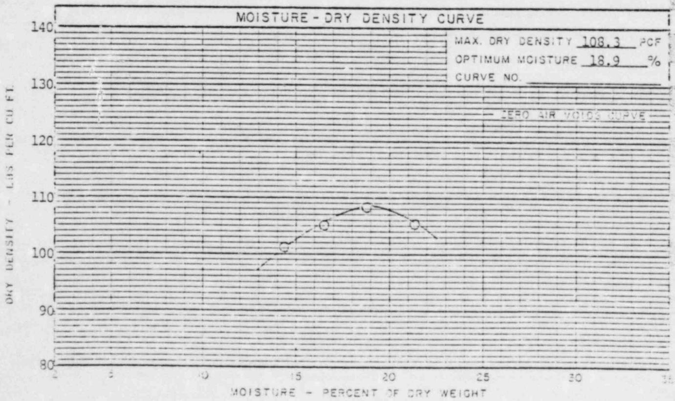
COMPACTION TEST PROCEDURE ASTM-D-698-78 METHOD A
