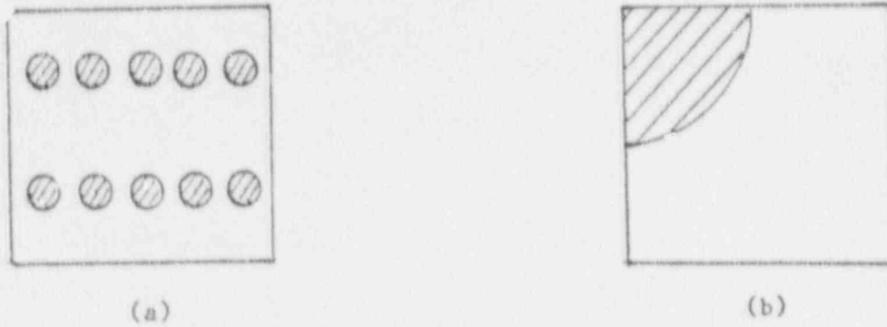
Fig. 18. Modeling (a) multiple structures or (b) fraction of a structure as one thermal structure
