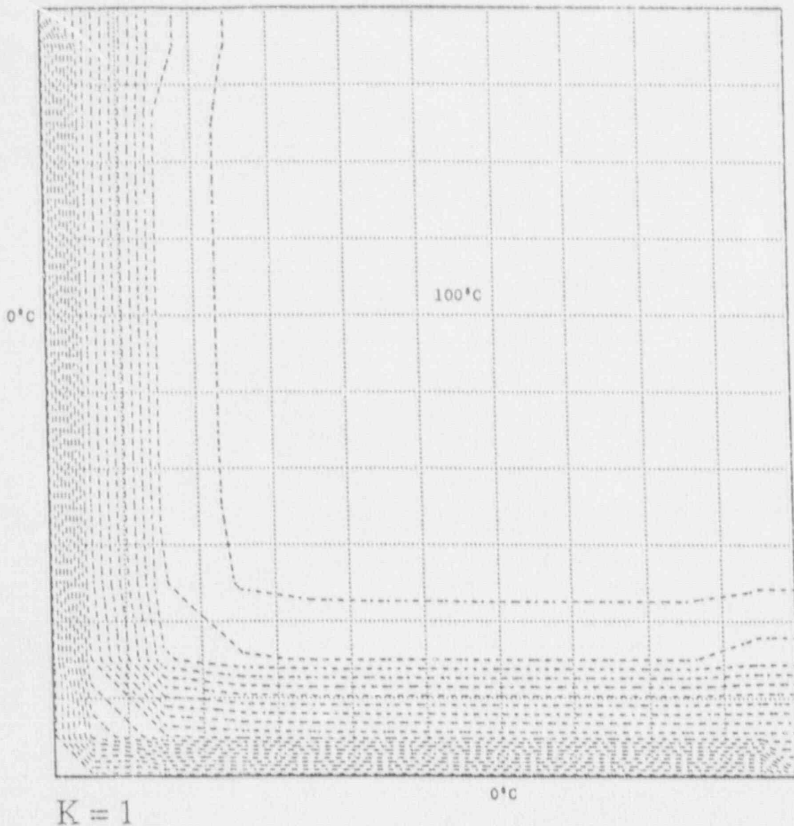
Fig. 30. Isotherms at lowest elevation ( k = 1 ) of a three-dimensional flow with m_x = m_y = m_z (FMSUD)
