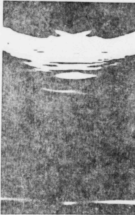
Fig. 3. Directed-beam B-scan image of a target block (SN4) with a concave surface and two round-bottom holes spaced 7.62 mm on center. The horizontal direction is parallel to the transducer scan line and the vertical direction is into the target block.
