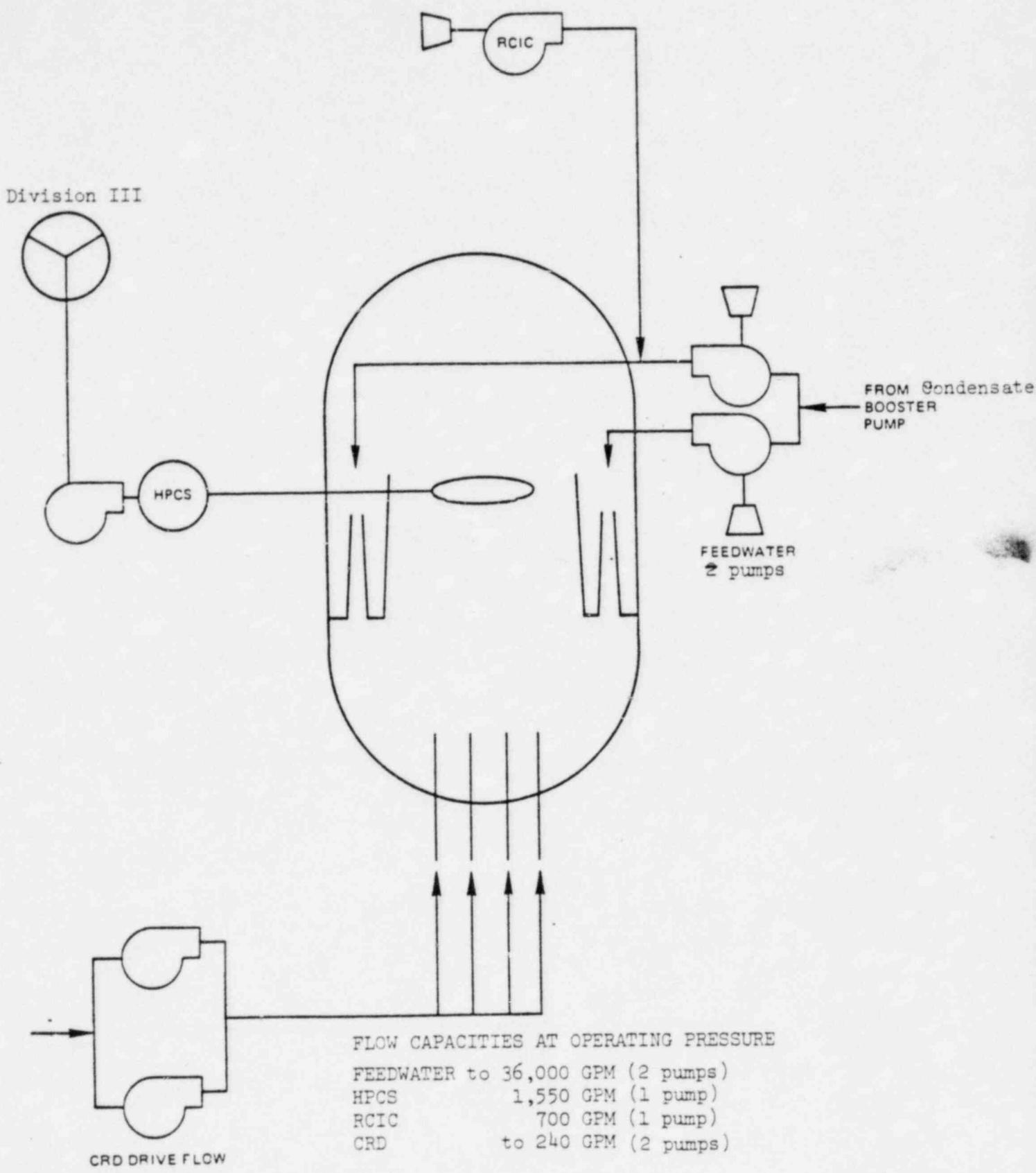
Figure 2.1.1-2. Typical 238 BWR/6 High Pressure Water Delivery Sources
