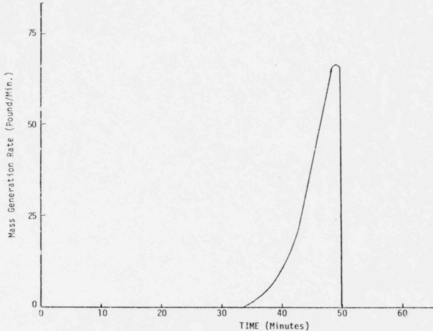
Figure 3.2.3-4 Hydrogen Mass Generation Rate vs. Time (Isolation with Delayed Water Makeup).
