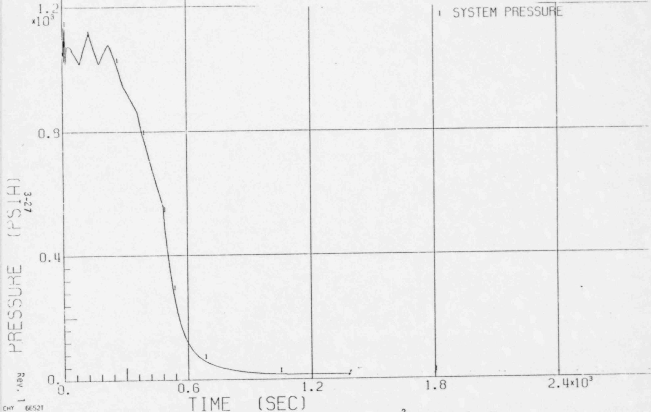
Figure 3.4.2-1 Reactor Pressure Transient for 0.1 Ft<sup>2</sup> Liquid Break with Temporary Failure of all Water Makeup.
