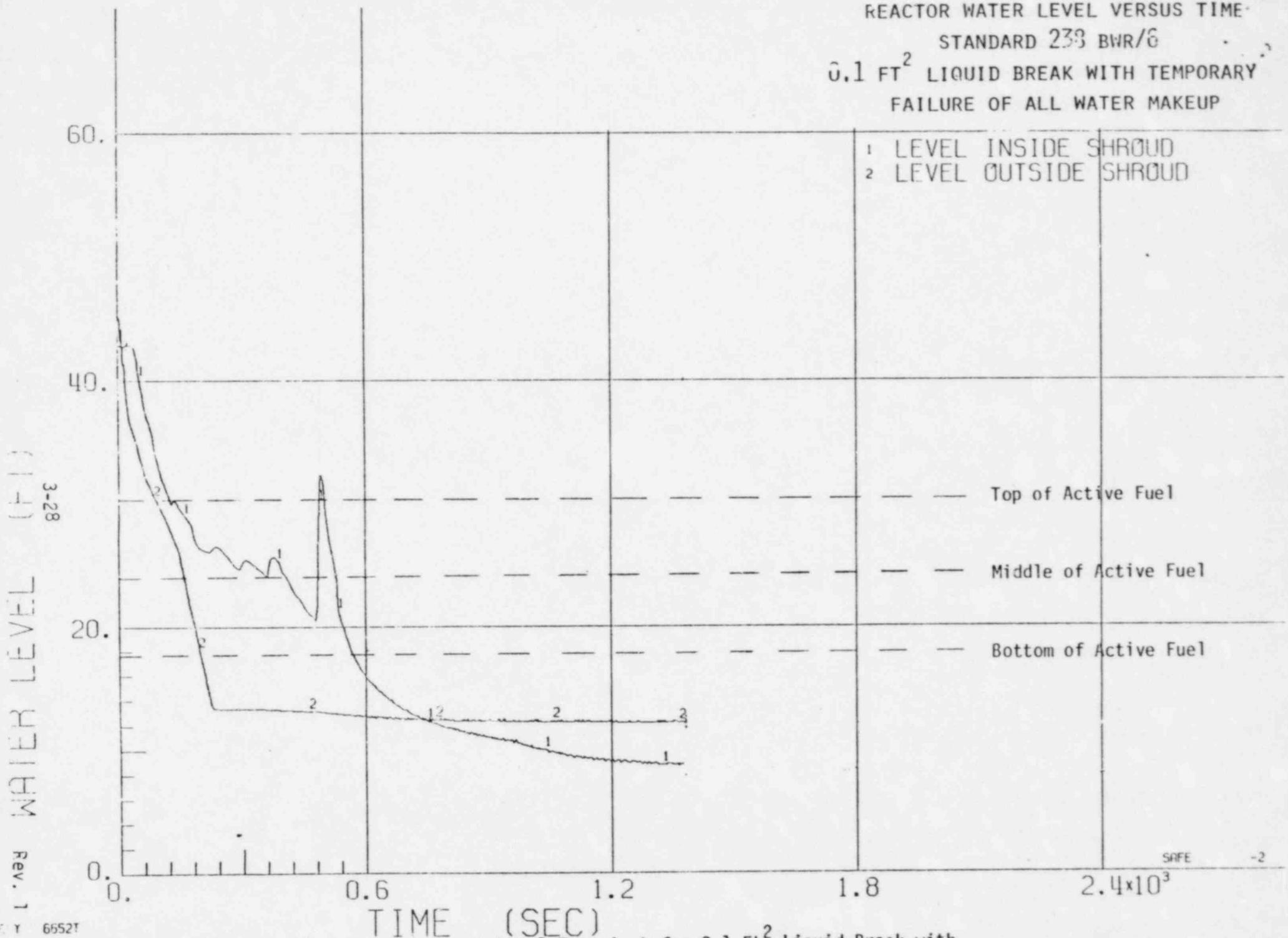
Figure 3.4.2-2 Reactor Water Level Transient for 0.1 Ft<sup>2</sup> Liquid Break with Temporary Failure of All Water Makeup.
