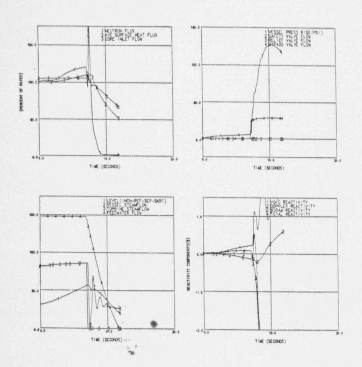
Figure 3. Plant Response to Feedwater Controller Failure
