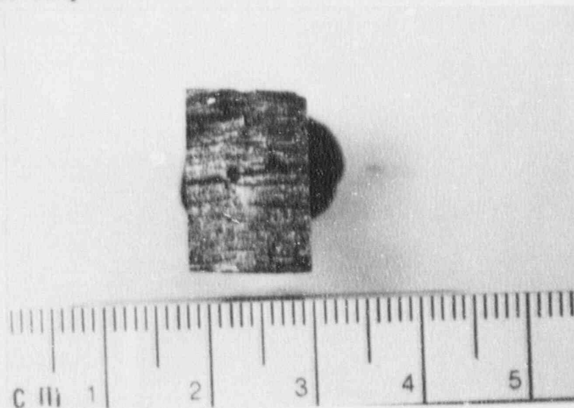
Figure 2. The portion of the boat-shaped sample after it was sectioned at SRI for the FRASTA evaluation.
