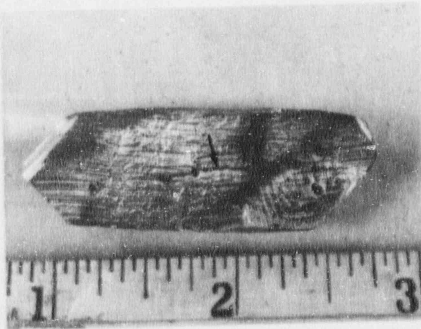
Figure 1. The boat-shaped sample as-removed from the 1A S/G at Zion Station. The arrow indicates the location of the surface flaw. Note the extent of pitting attack on the surface of the sample.
