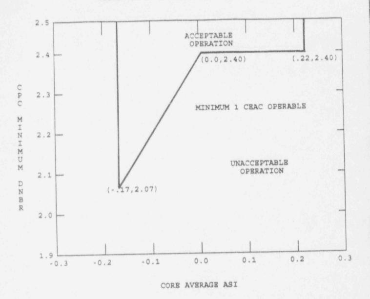
DNBR MARGIN OPERATING LIMIT BASED ON CORE PROTECTION CALCULATORS (COLSS OUT OF SERVICE, CEACS OPERABLE)
