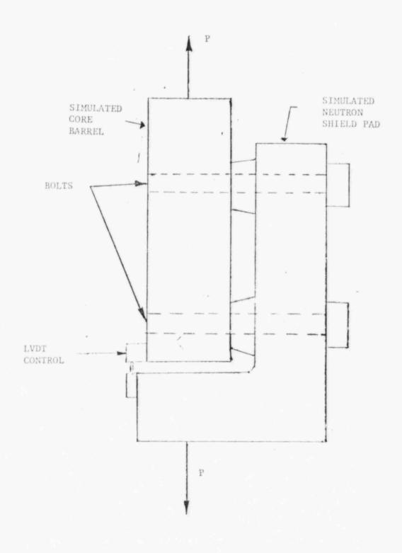
FIGURE A-1. NEUTRON SHIELD BOLT ASSEMBLY SIDE VIEW
