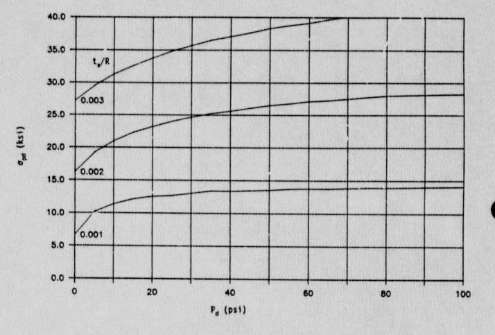
Figure 7-8. Compressive Axial Stress Capacity For Vertical Tanks, Diamond-Shape Buckling (Steel, E = 30,000 psi) (Source: Reference 26, Figure 2.10)
