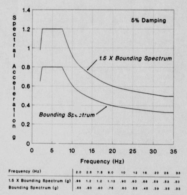
Figure 4-2. Seismic Capacity Bounding Spectrum Based on Earthquake Experience Data (Source: Reference 5)
