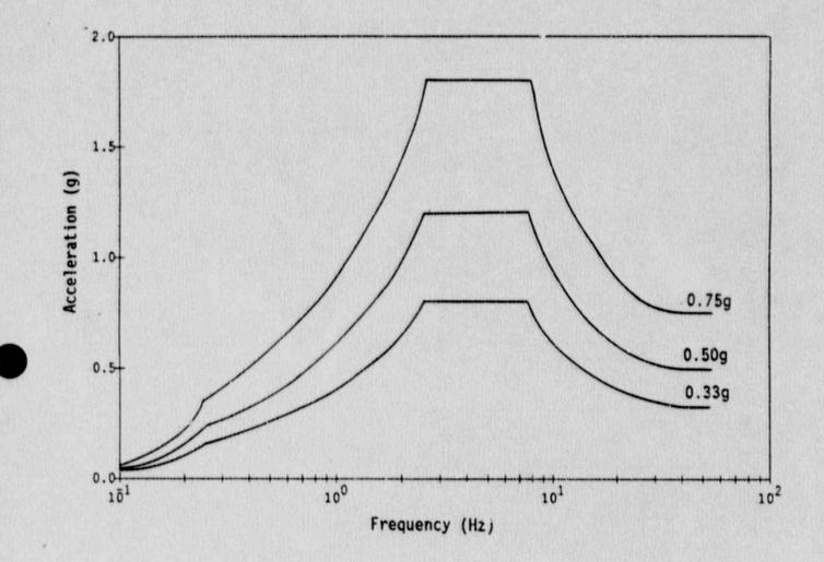
Figure 8-9. Rod Fatigue Bounding Spectrum Anchored to 0.33g, 0.50g, and 0.75g. (Source: Reference 9)
