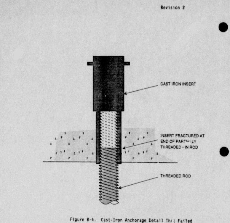
gure 8-4. Cast-Iron Anchorage Detail Thrt Failed at the Pacific Bell Alhambra Station, 1987 Whittier Earthquake. (Source: Reference 9)
