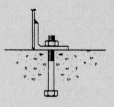
D Desirable Stiff Bolted Anchorage Structural angle base provides adequate stiffness.
