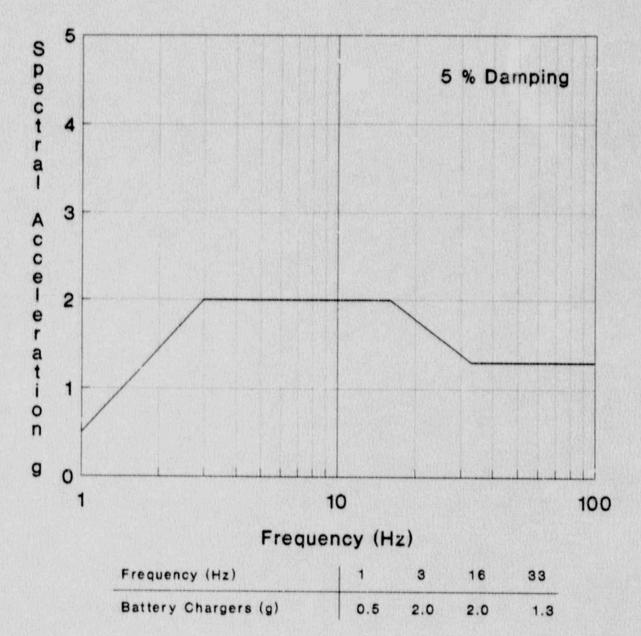
Figure B.16-1. Generic Equipment Ruggedness Spectra (GERS) for Battery Chargers. (Source: Reference 6)
