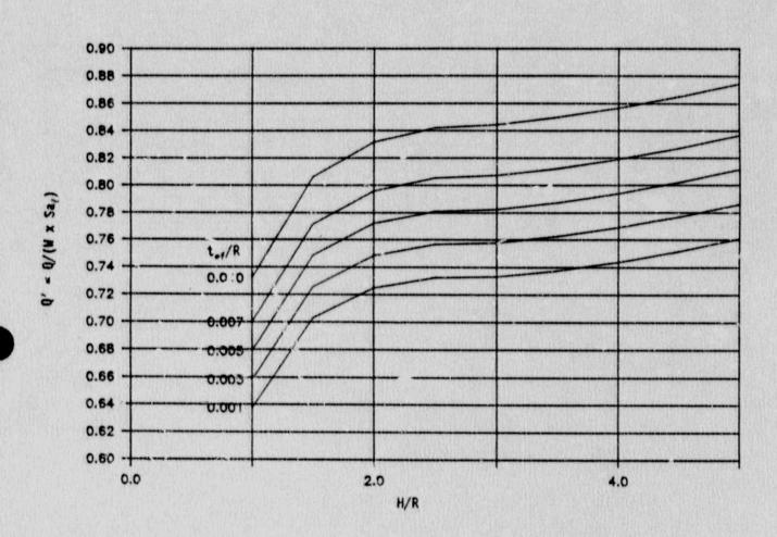
Figure 7-3. Base Shear Load Coefficient For Vertical Tanks (Source: Reference 26, Figure 2.3)
