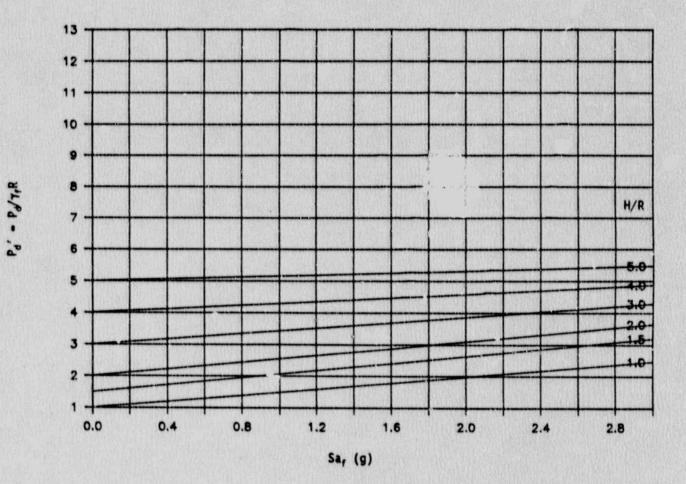
igure 7-7. Pressure Coefficient For Diamond-Shape Buckling
