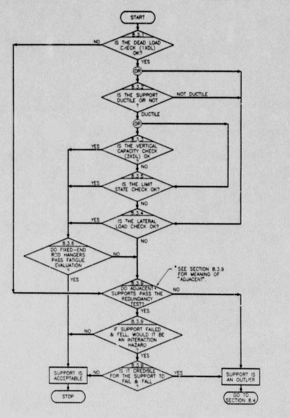
Figure 8-6. Logic Diagram for Limited Analytical Review of Suspended Raceway Supports.
