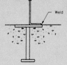
A Undesirable Flexible Welded Anchorage Uplift causes sheet metal frame to bend.
