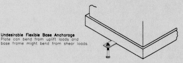
Figure 4-5. Examples of Stiff and Excessively Flexible Anchorage Connections. (Source: Reference 5)
