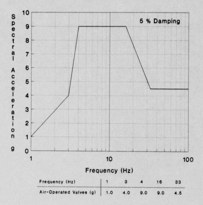
Figure B.7-3. Generic Equipment Ruggedness Spectra (GERS) for Air-Operated Valves. (Source: Reference 6)
