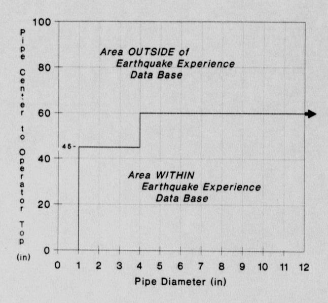
Figure B.7-1. Valve Operator Cantilever Length Limits for Air-Operated Diaphragm Valves, Spring-Operated Pressure Relief Valves and Piston-Operated Valves of Light-Weight Construction. (Source: Reference 5)
