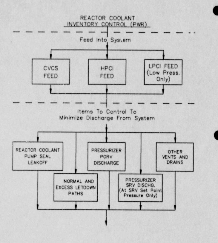
Figure A-4. Safe Shutdown Alternatives for Reactor Coolant Inventory Control of PWRs. Discharge from the Reactor Coolant System (PWR). There are several paths through which reactor coolant can leave the reactor coolant system. Listed below are typical discharge paths which should be controlled to minimize loss of inventory:
