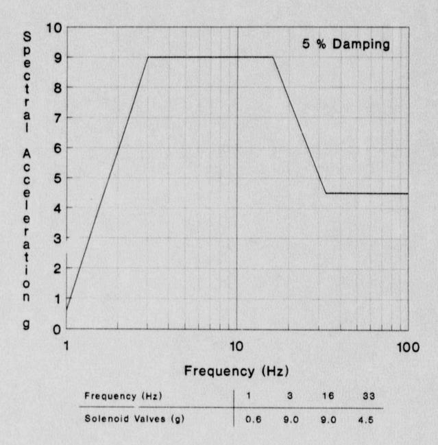
Figure B.8-3. Generic Equipment Ruggedness Spectra (GERS) for Solenoid-Operated Valves. (Source: Reference 6)
