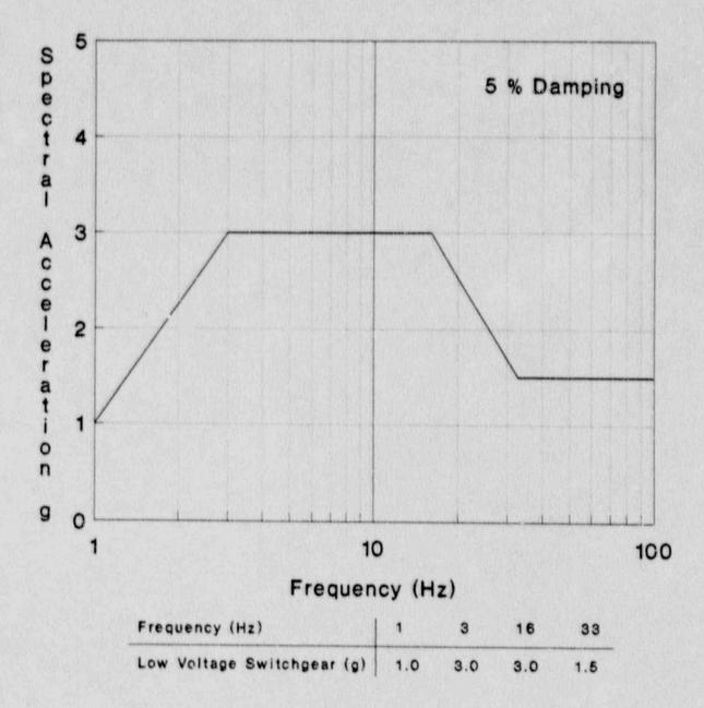
Figure B.2-1. Generic Equipment Ruggedness Spectra (GERS) for Low Voltage Switchgear. (Source: Reference 6)
