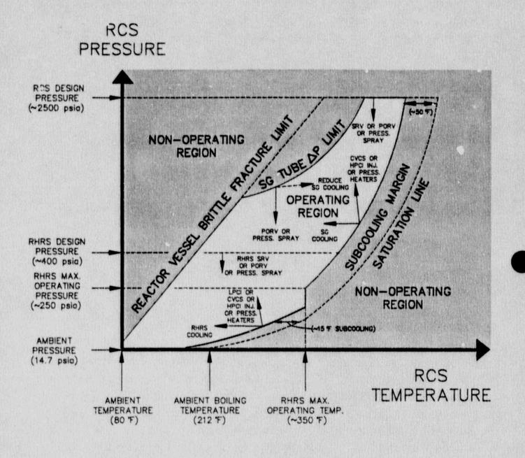
Figure A-3. Pressure-Temperature Limits For Typical PWR Reactor Coolant System Without Reactor Coola.t Pumps Operating. auxiliary pray system. (Normal spray is not available since the reactor coolant pumps are not running due to the assumed loss of offsite power.)
