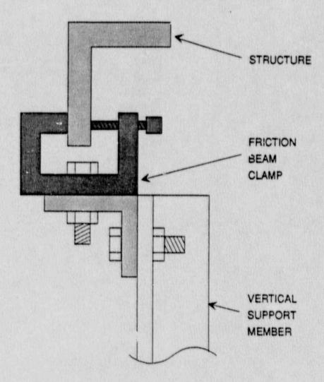
Note: This arrangement may loosen and slip, resulting in support collapse.
