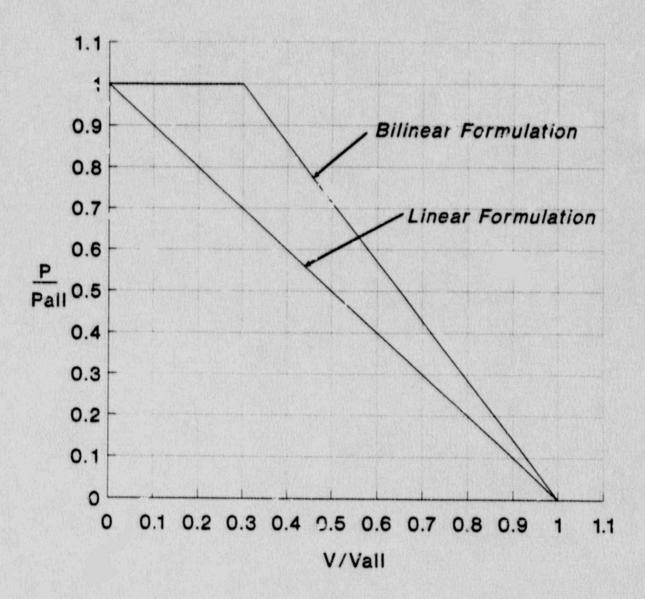
Figure C.2-4. Shear-Tension Interaction Limitations for Expansion Anchors (Source: Reference 7)
