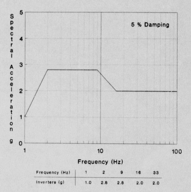
Figure B.16-2. Generic Equipment Ruggedness Spectra (GERS) for Inverters. (Source: Reference 6)
