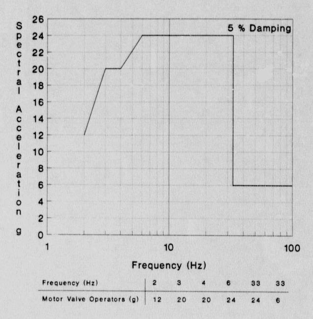
Figure B.8-2. Generic Equipment Ruggedness Spectra (GERS) for Motor Valve Operators. (Source: Reference 6)
