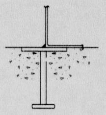
C Desirable Stiff Welded Anchorage Loads ross through sheet metal wall.
