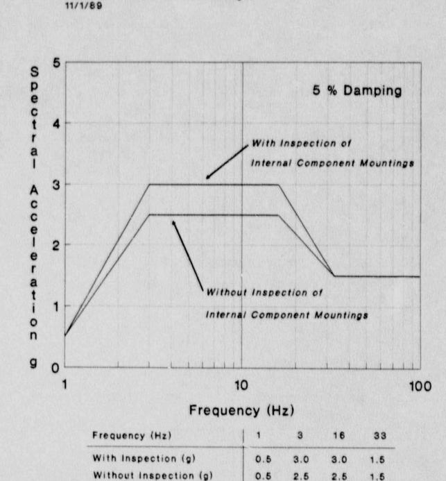
Figure B.3-1. Generic Equipment Ruggedness Spectra (GERS) for Medium Voltage Switchgear. (Source: Reference 5)
