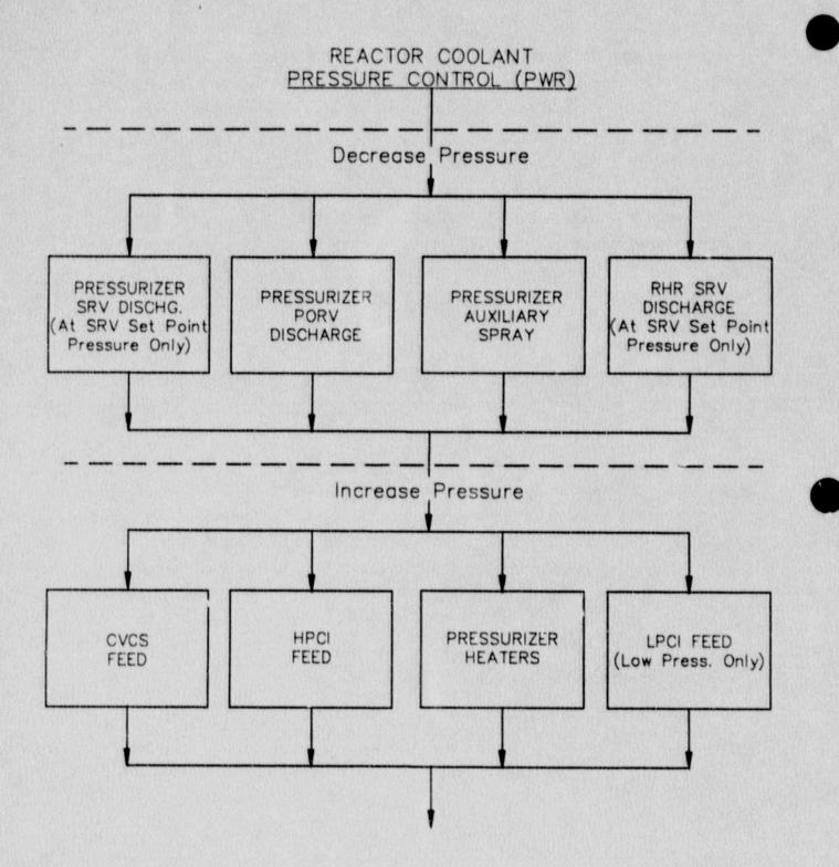
Figure A-2. Safe Shutdown Alternatives for Reactor Coolant Pressure Control of PWRs.
