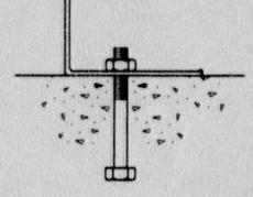
B Undesirable Flexible Bolted Anchorage Uplift couses sheet metal to bend.
