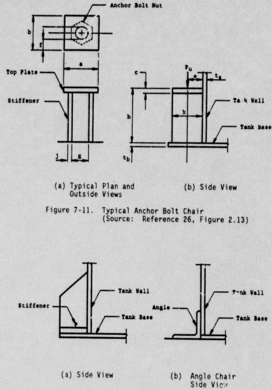
Figure 7-12. Alternate Ancho" Bolt Chairs (Source: Reference 26, Figure 2.14)
