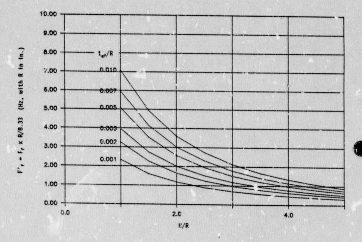
Figure 7-2. Fluid-Structure Impulsive Mode Frequency Coefficient for Vertical Carbon Steel Tanks Containing Water. (Source: Reference 26, Figure 2.3)
