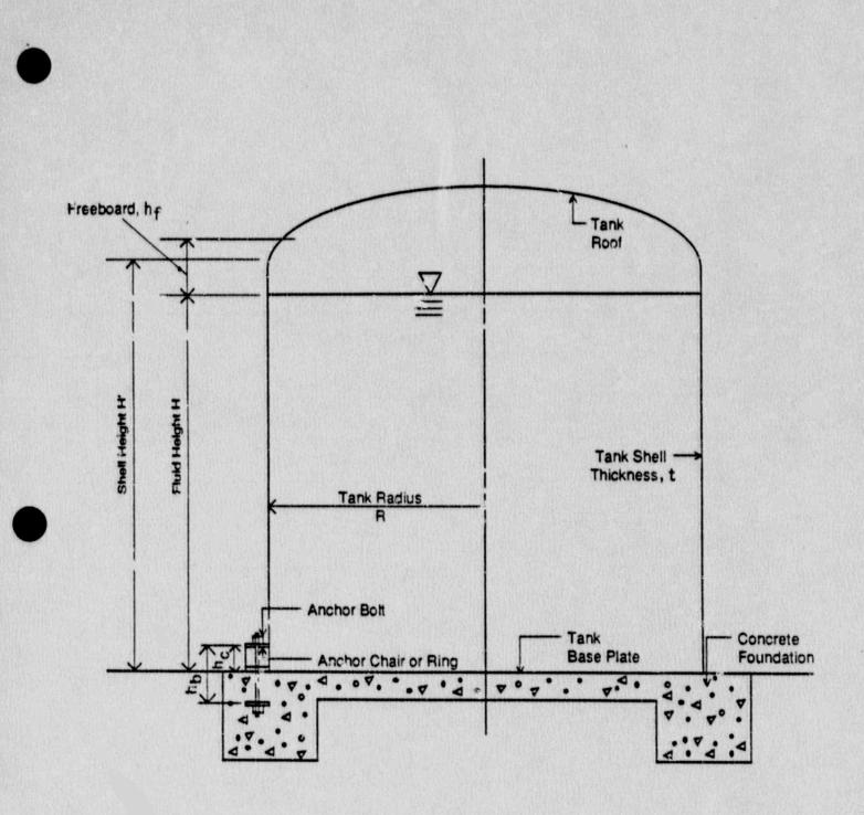
Figure 7-1. Large Vertical Tank (Source: Reference 26, Figure 2.1)
