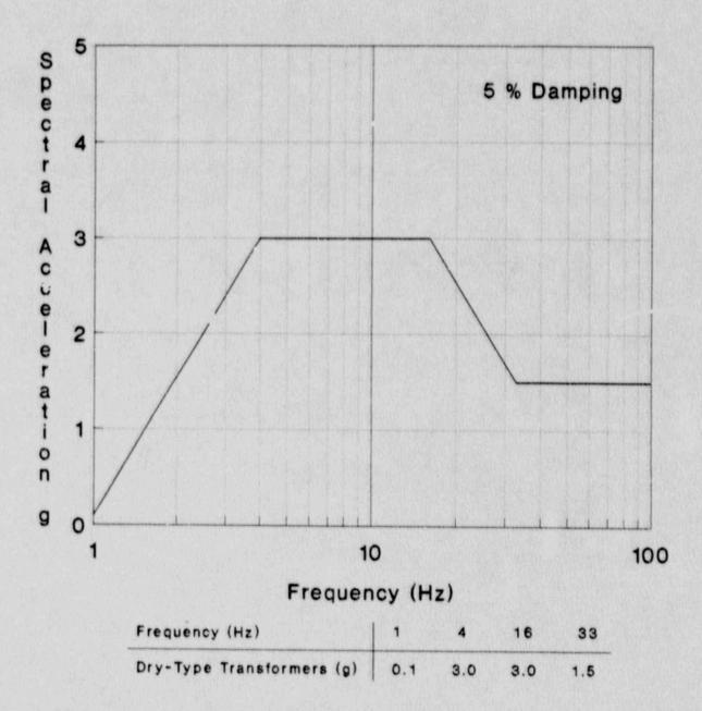
Figure B.4-1. Generic Equipment Ruggedness Spectra (GERS) for Dry-Type Transformers. (Source: Reference 6)
