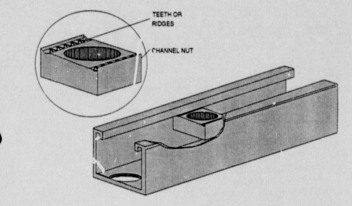
Figure 8-1. Channel Nut With Teeth or Ridges in Light Metal Framing Strut. (Source: Reference 9)
