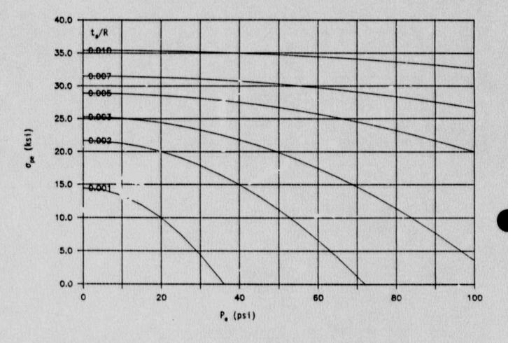
Figure 7-6. Compressive Axial Stress Capacity For Vertical Tanks, Elephant-Foot Buckling (Steel, E = 30,000 psi,  $\sigma_y$  = 36,000 psi) (Source: Poference 26, Figure 2.8)
