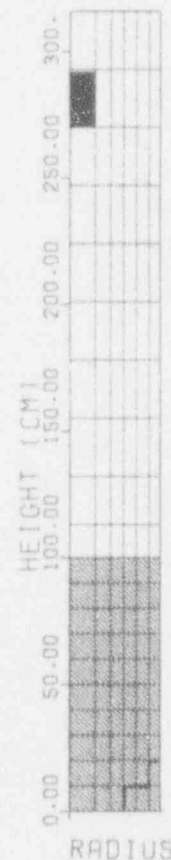
Figure 1: FARO LWR 2nd Quenching Test; geometry, calculational mesh and initial material distributions assumed for the calculations. The radius of the vessel is 35.5 cm.
