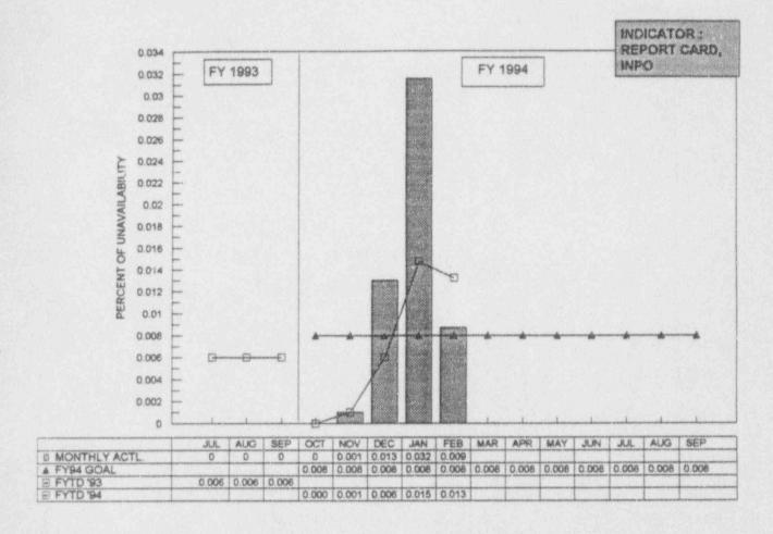
ANALYSIS: THERE WERE TWO PLANNED ACTIVITIES THIS MONTH. ONE WAS ON THE 2A-A CCP FOR 5.25 HOURS AND ONE WAS ON THE 2AA RHR PUMP FOR 18.18 HOURS TO REPAIR A CCS SEAL LEAK, CLEAN THE MOTOR COOLER SCREEN, AND REPAIR AN INDICATOR ON 2-74-520.
