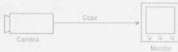
Figure 5-2. CCTV alarm assessment system using coax cable
