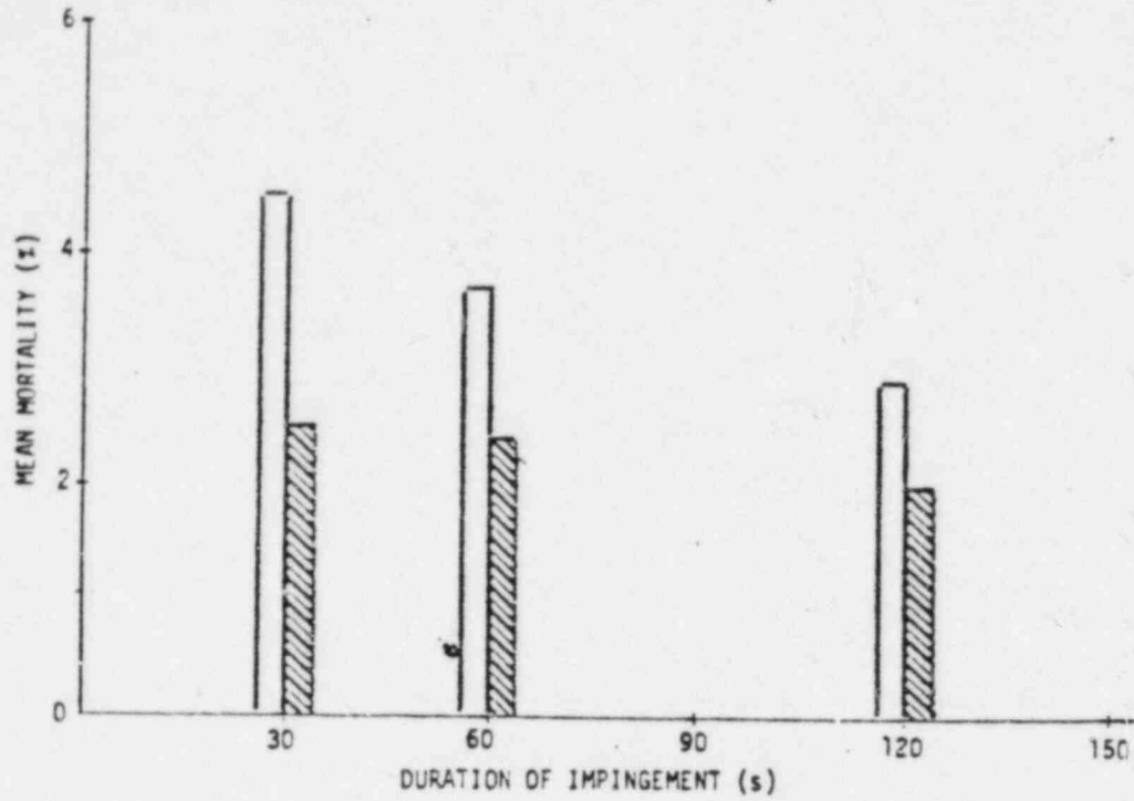
Fig. 7. Mortality of Striped Bass Eggs Due to Impingement on Screen P2A at an Approach Velocity of 15.24 cm/s. Cross-hatched bars indicate controls.
