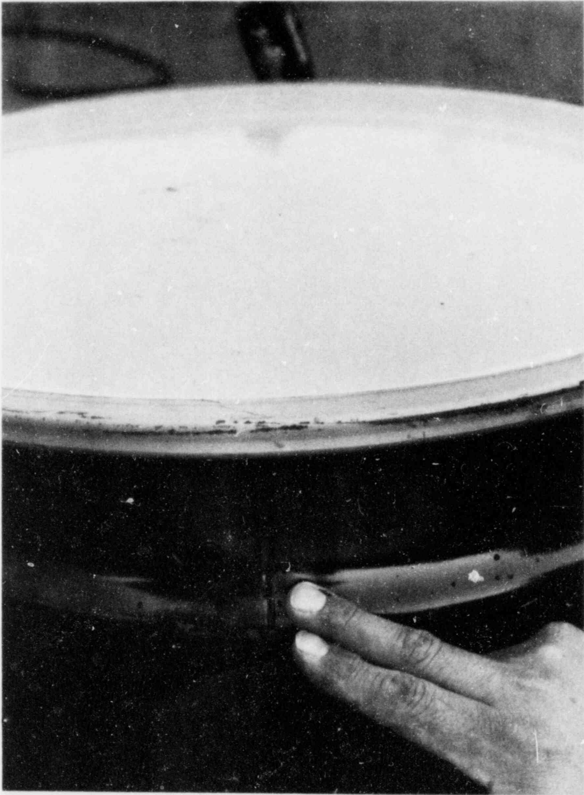
Figure 5.3 Butt weld on DOT 17H causing failure to sustained pressure.
