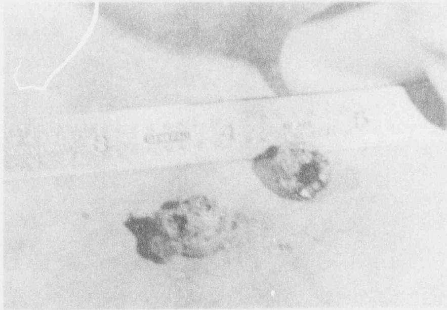
Fig. 3-52 Hollow Particles from the Debris Bed for Experiment CCM-5
