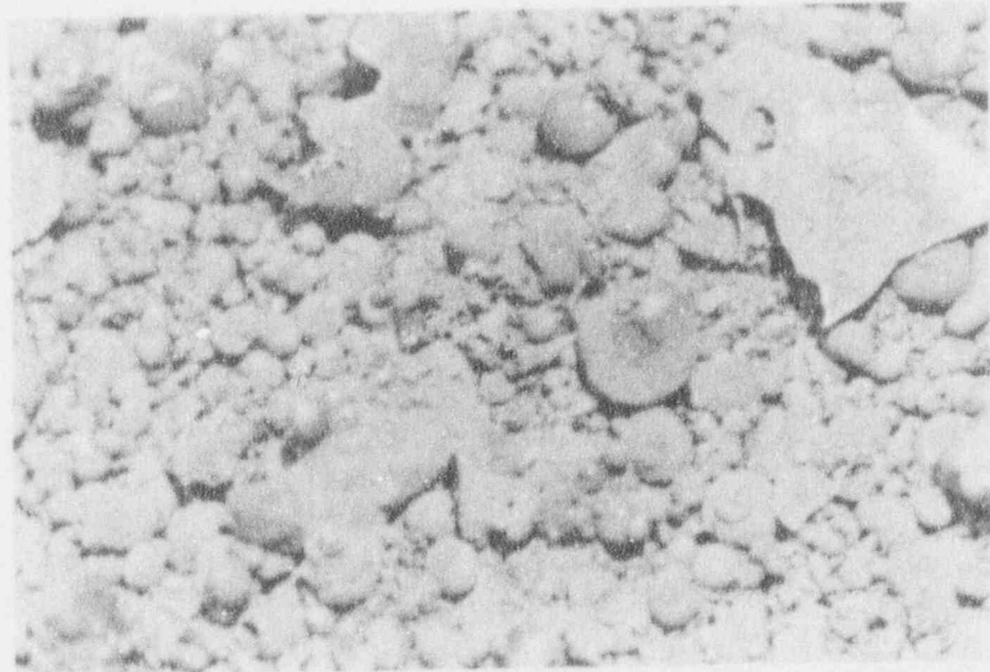
Fig. 3-56 Surface of the Debris Bed in Experiment CCM-6
