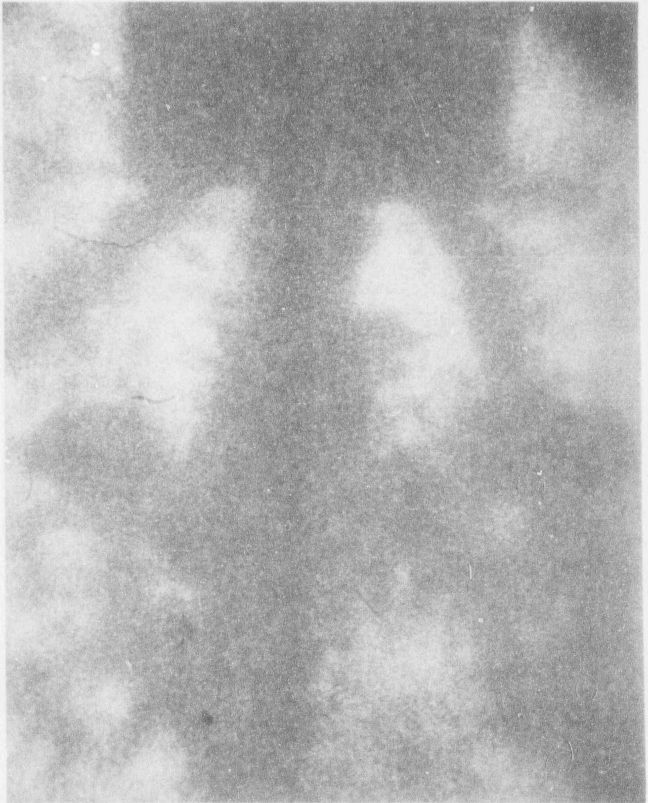
Fig. 3-7 X-Ray Photography of Corium Jets Emerging from the Impingement Holes for Experiment CCM-2
