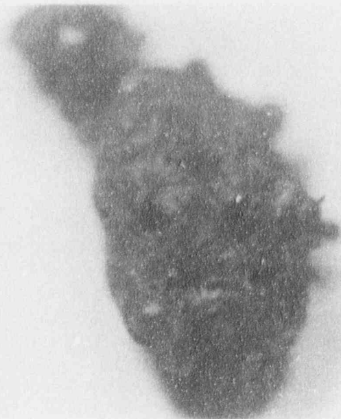
Fig. 3-38 Oblong Debris Particle with Holes from the CCM-3 Interaction Vessel Base
