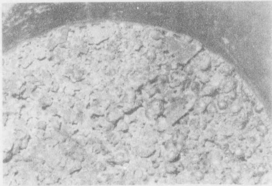
Fig. 3-13 View of Debris in the Bottom of the Thermite Vessel Used in Experiment CCM-1
