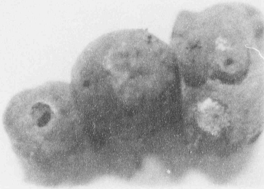
Fig. 3-37 Agglomerated Debris Particle from the CCM-3 Interaction Vessel Base
