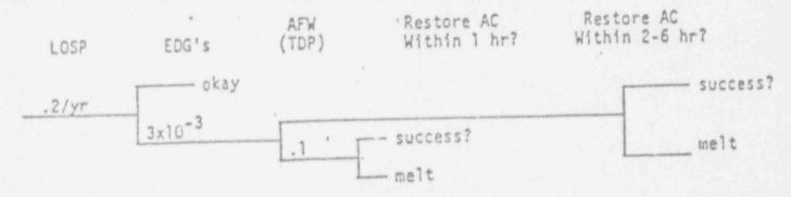
Blackout with successful auxiliary feedwater (turbine driven pump) can be expected at a frequency of roughly  $6 \times 10^{-4}$ /yr. The turbine driven AF pur, has a finite success window, however. One of several factors will lead to core melt if AC power is not ultimately restored. These factors include: (a) loss of reactor coolant inventory (blown RCP seals, etc.); (b) dead batteries (discharge or overheat); (c) high pump room temperatures (no HVAC); or (d) depletion of condensate.
