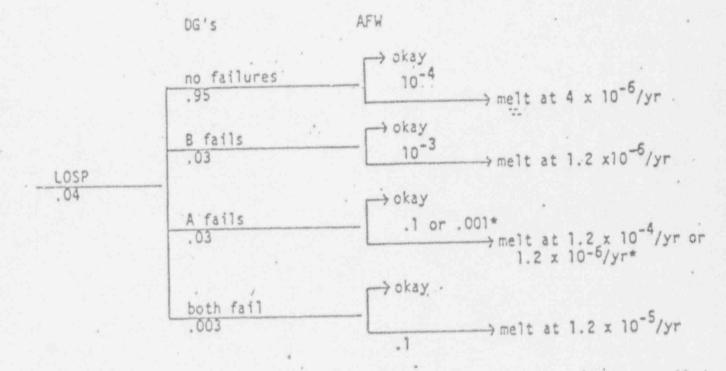
\*The higher failure rate applies if one of the diesel generators (we have called it B) cannot power a motor driven AFW train; the lower failure rate applies if both diesel generators can power a motor driven AFW train.
