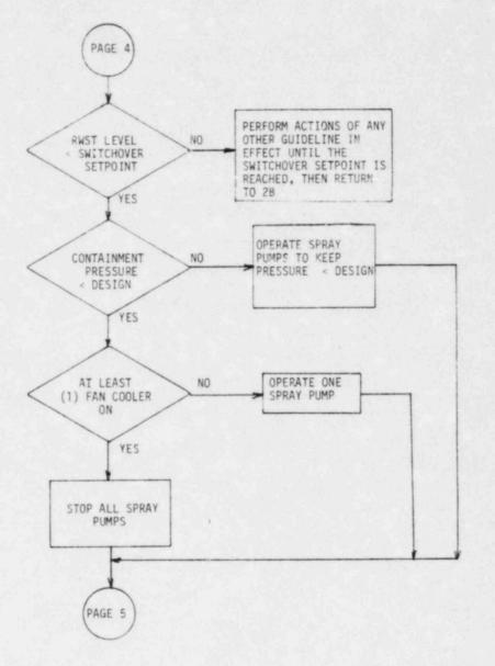
NUMBER OF FAN COOLERS REQUIRED TO MAINTAIN PRESSURE BELOW CONTAINMENT DESIGN PRESSURE.
