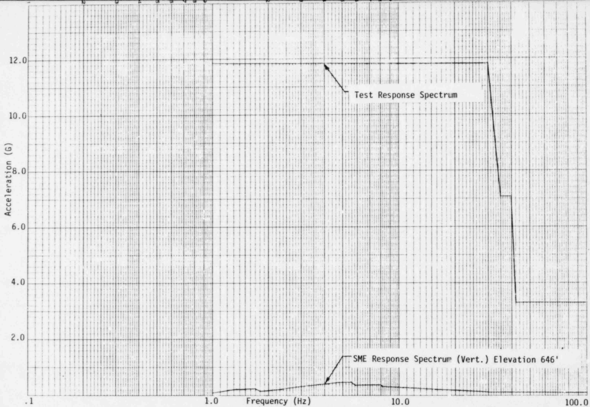
FIGURE VII-A-11-3. COMPARISON OF 3% DAMPED SME SPECTRA WITH TEST RESPONSE SPECTRA FOR MIDLAND CHILLER CONTROL PANELS
