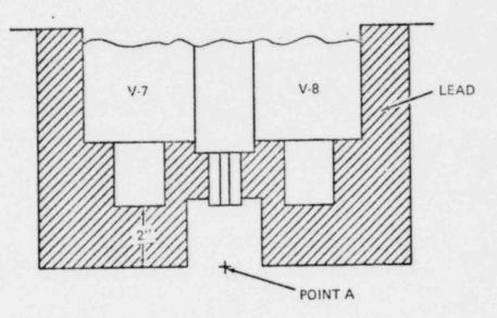
Dose rate at point A is comprised of dose rate 2 in. from the end of needle guide plus dose rate 2 in. from the end of valves V-7 and V-8, shielded by 2 in. of lead which has a shielding factor of 0.0381.
