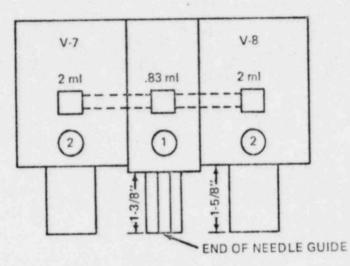
Assume shielding factor for brass needle guide 1-3/8 in. long = 0.31.
