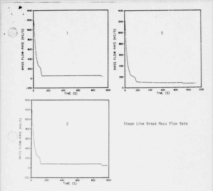
(1) SG isolated at 15 min (900 s) by closing of B loop isolation values. Mass flow does not go to zero because 9000 kg of primary water remains between the top of the u-tubes and the SGTR in the tube sheet. That water drains through the SGTR over the next 30 min.
