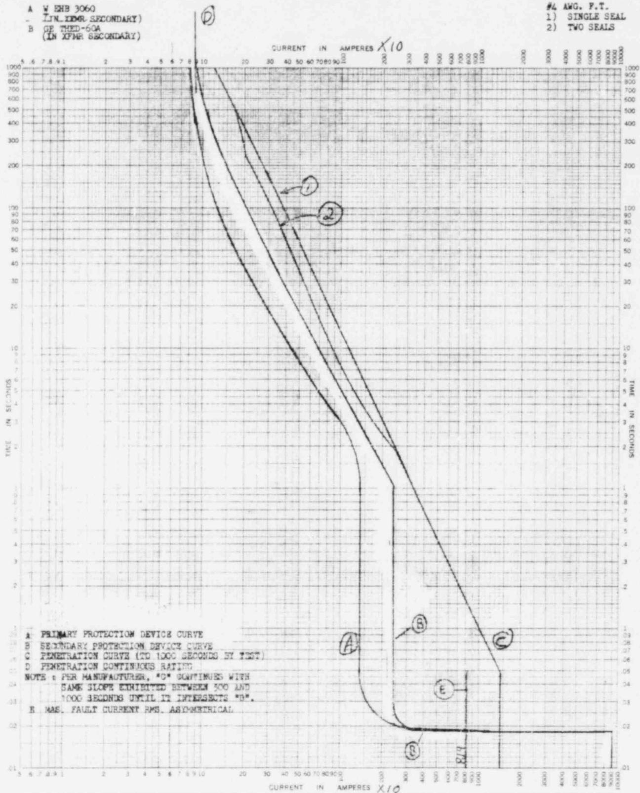
For \_\_\_\_\_ TIME-CURRENT CHARACTERISTIC CURVES
