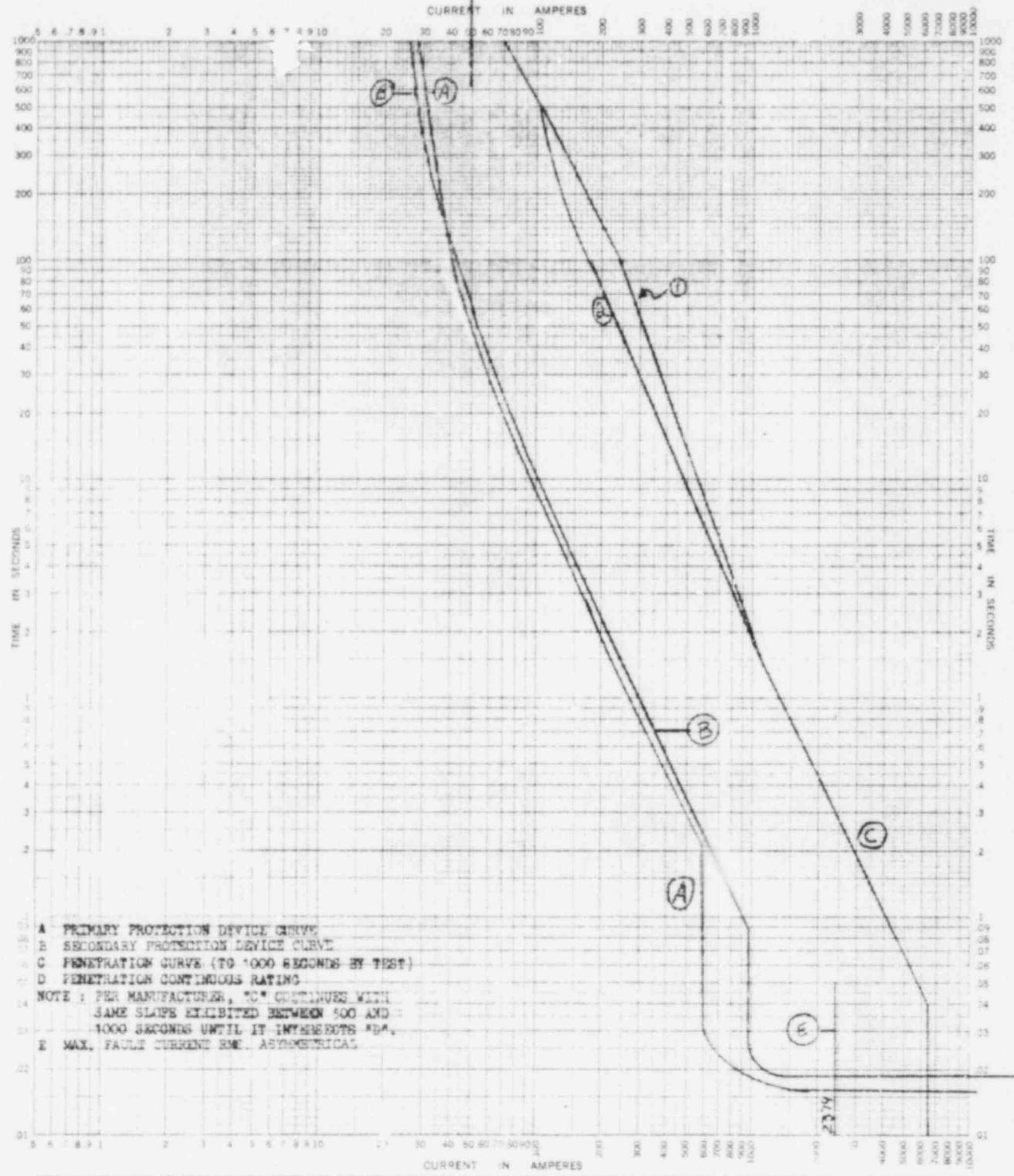
For \_\_\_\_\_ TIME-CURRENT CHARACTERISTIC CURVES
