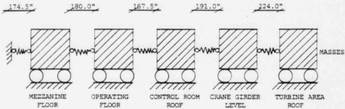
FIG. B.13 MECHANICAL MODEL 3 FOR VERTICAL ANALYSIS OF TURBINE BUILDING
