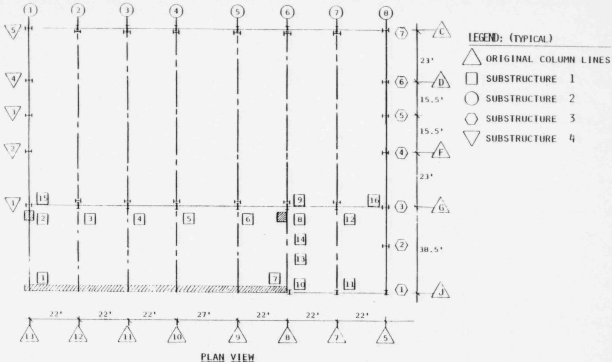
FIG. B.2 SUBSTRUCTURE MODELING
