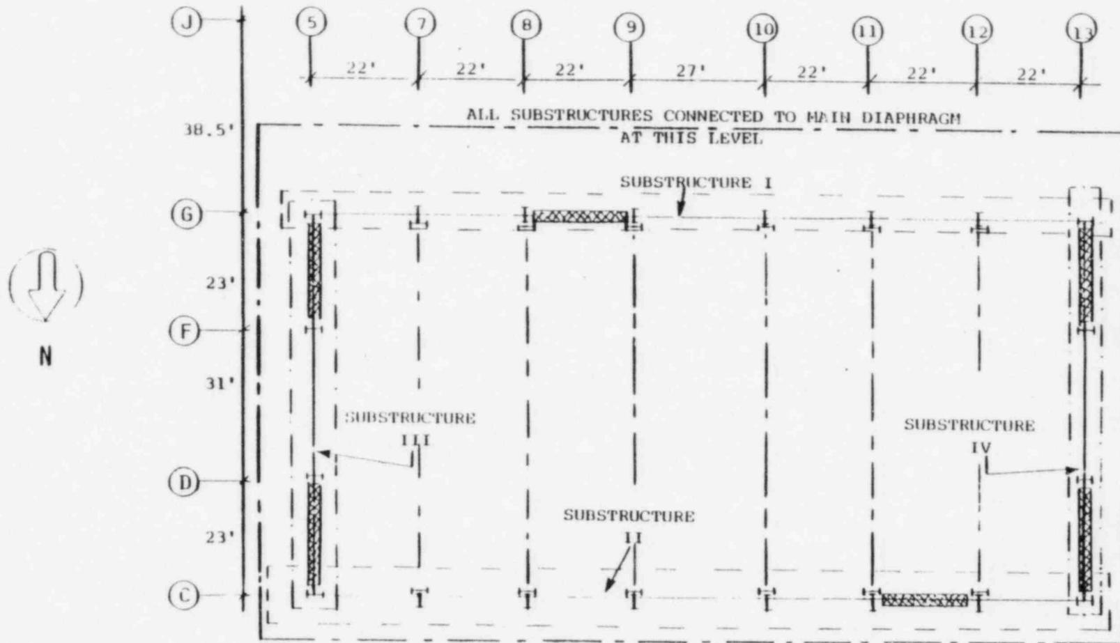
FIG. B.7 SUBSTRUCTURES AT ELEVATION 1096'
