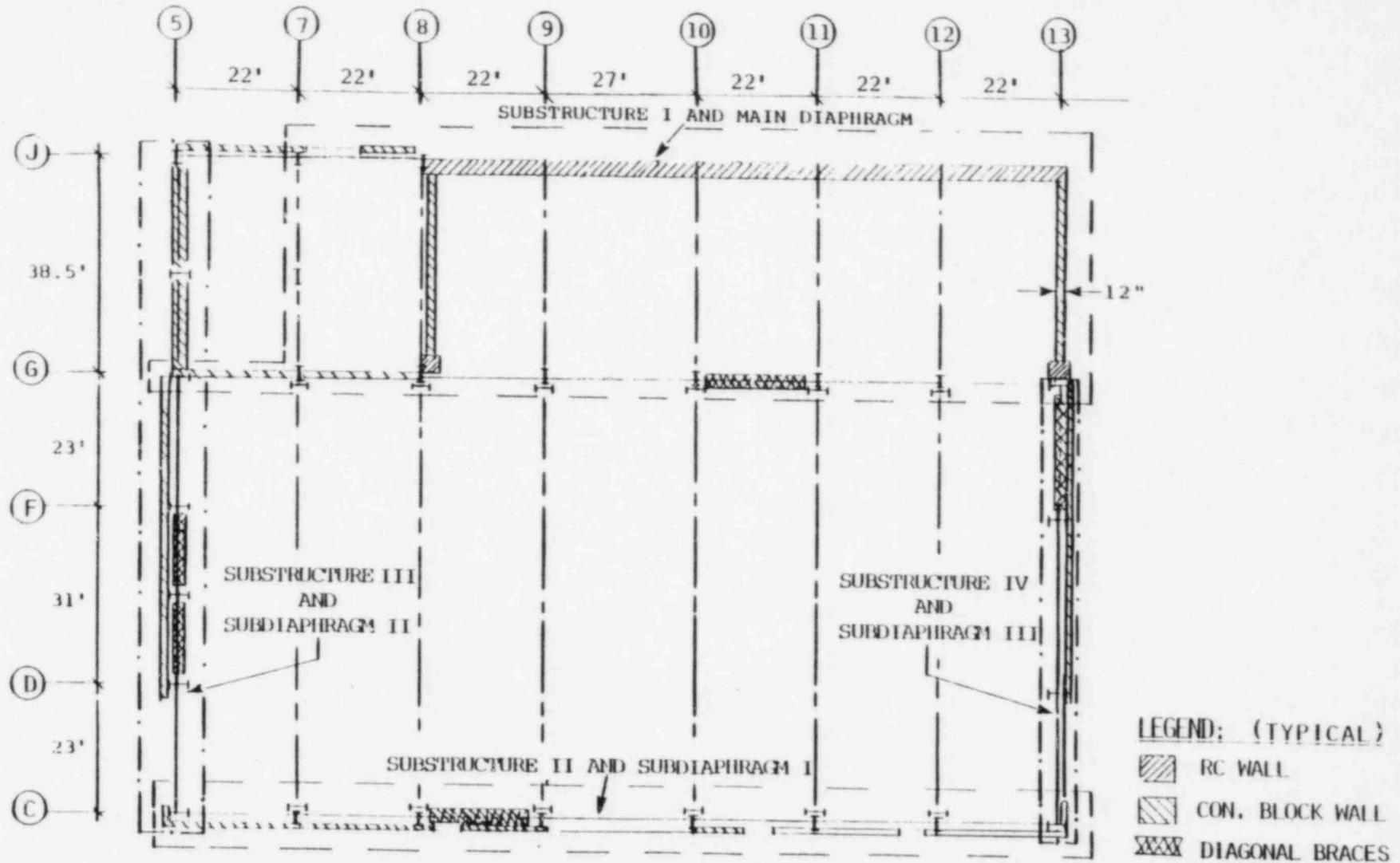
FIG. B.3 SUBSTRUCTURES AT ELEVATION 1037'-8"
