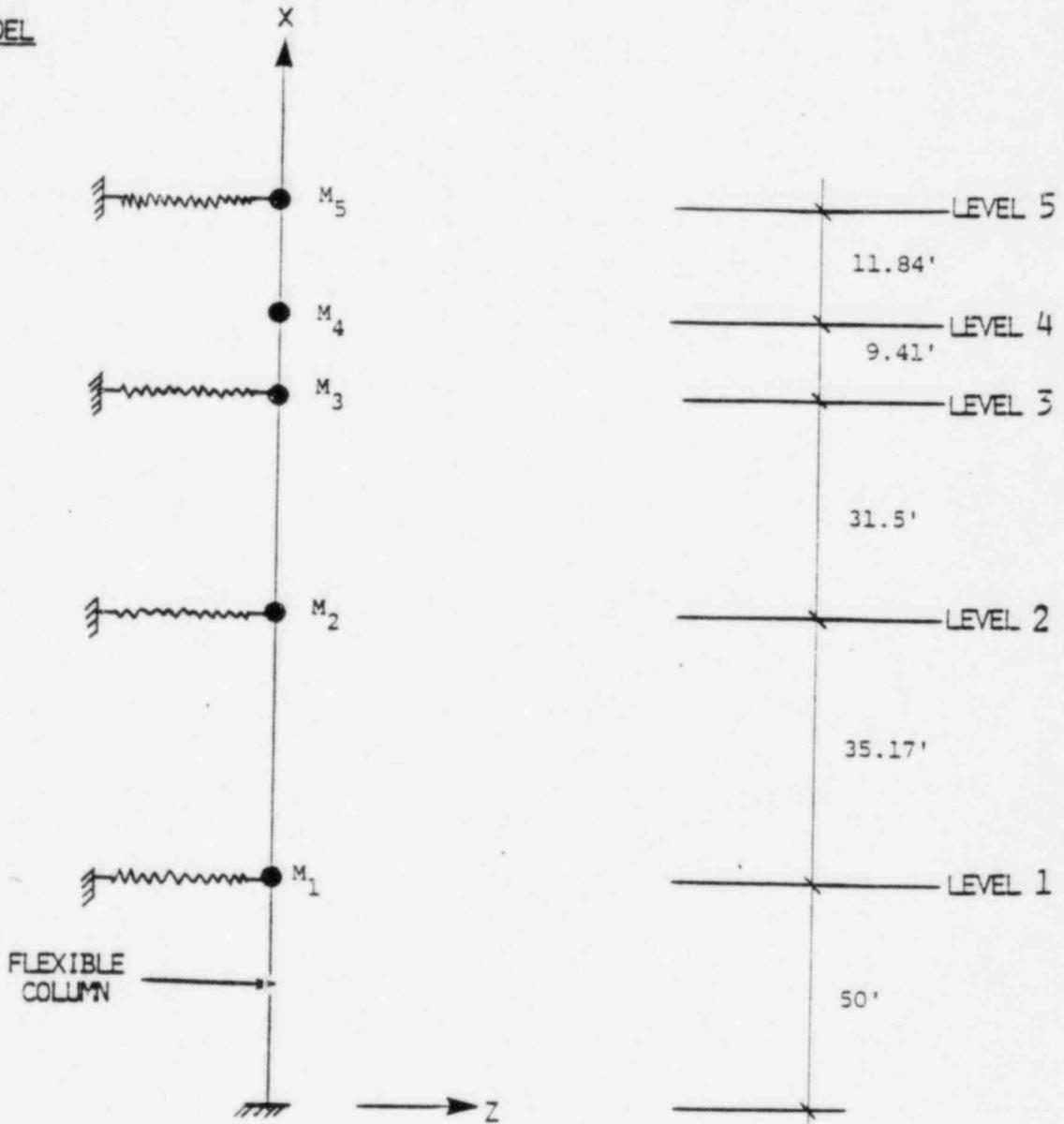
FIG. B.14 STICK MODEL FOR VERTICAL ANALYSIS OF TURBINE PEDESTAL
