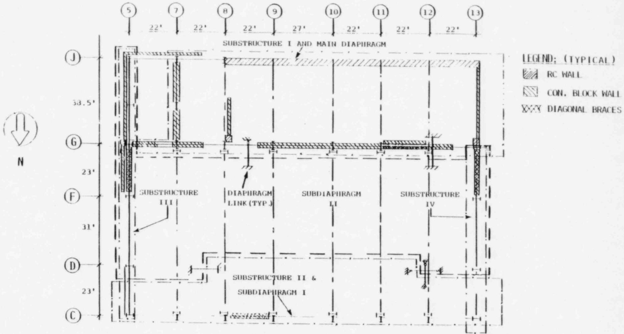
FIG. B.4 INTERCONNECTED FLOOR DIAPHRAGMS
