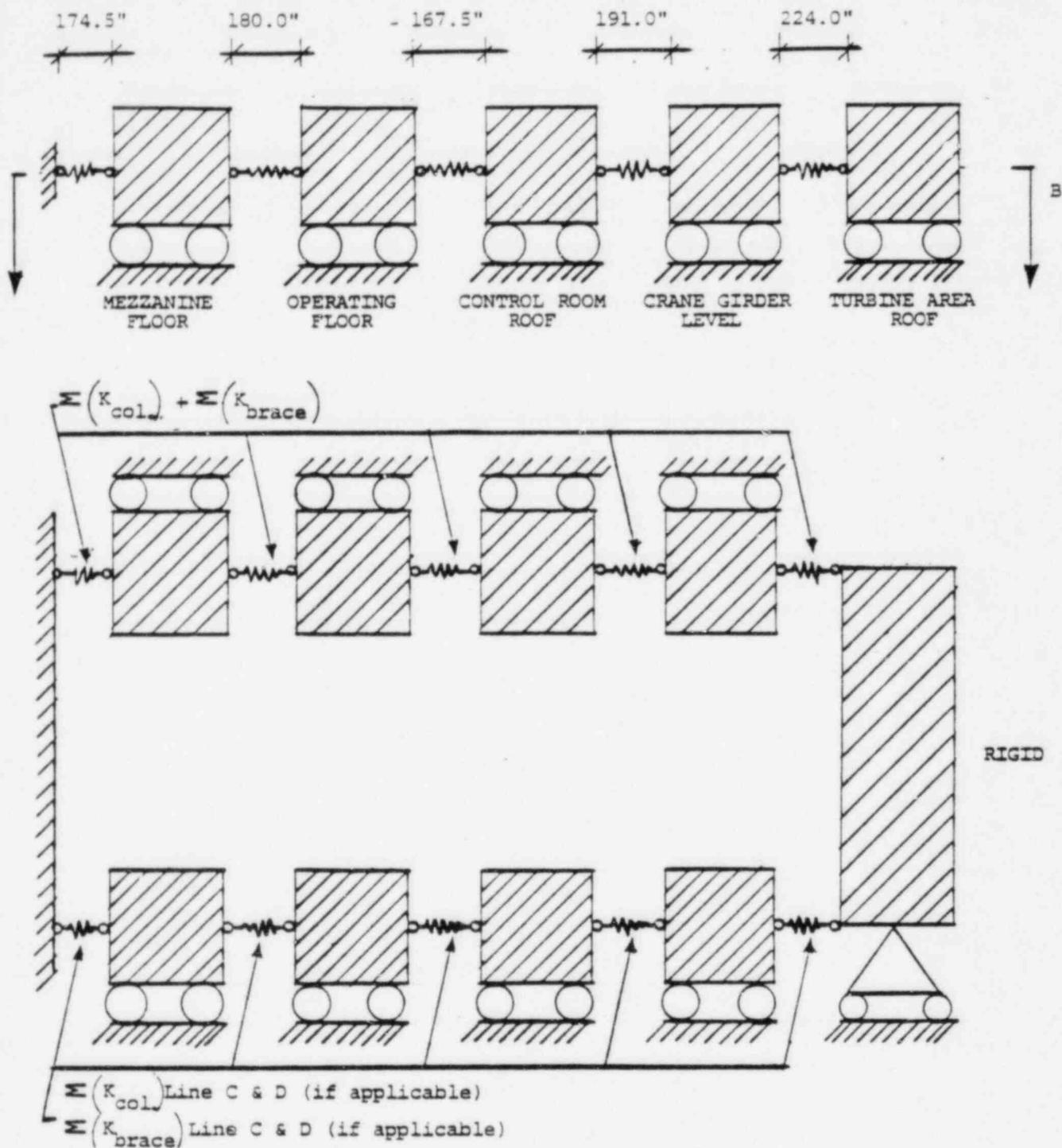
FIG. B.12 MECHANICAL MODEL 2 FOR VERTICAL ANALYSIS OF TURBINE BUILDING
