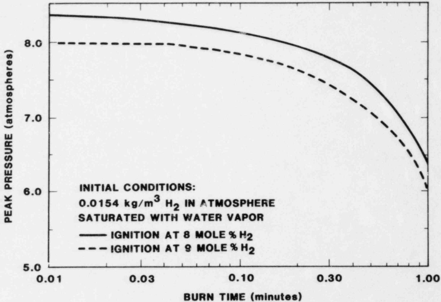
Figure 8.3.3-1. Effect of Hydrogen Combustion Burn Time on the Single Compartment Peak Pressure Predicted by HECTR for Zion With Three Containment Spray Trains Operating.
