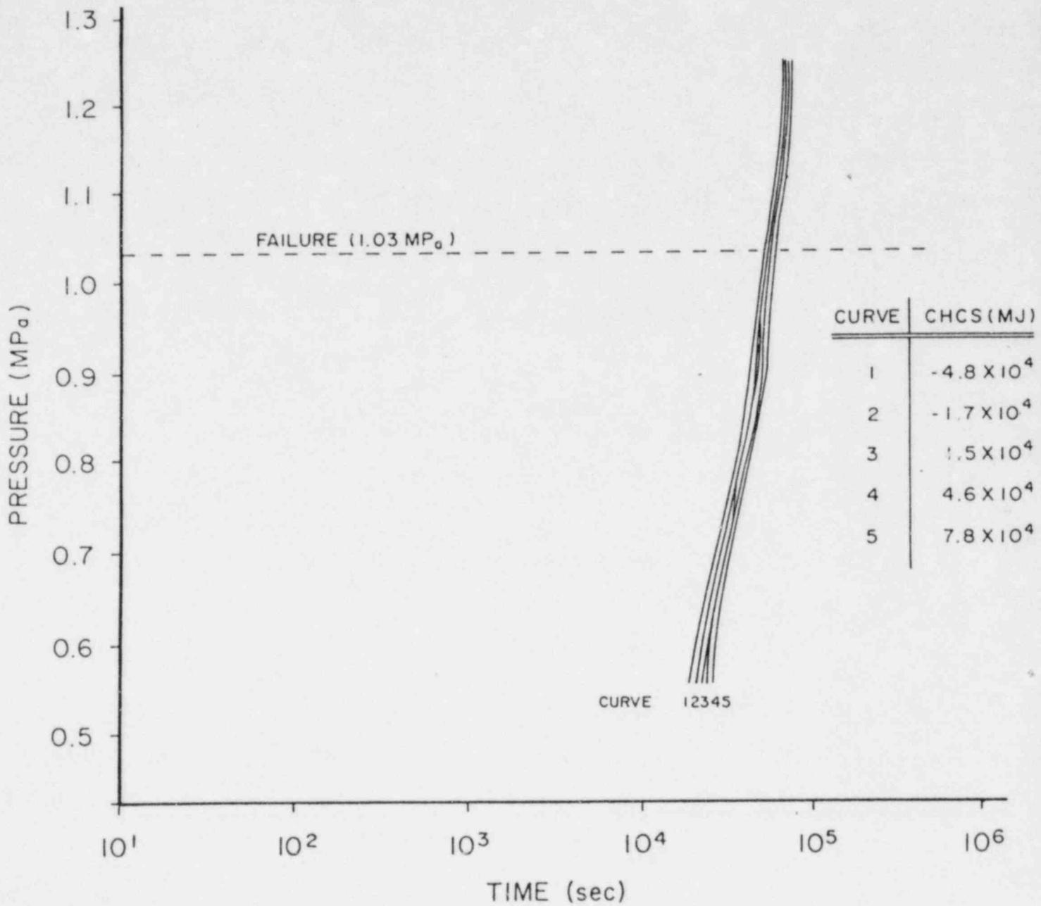
Figure C-2. Maximum Containment Pressurization
