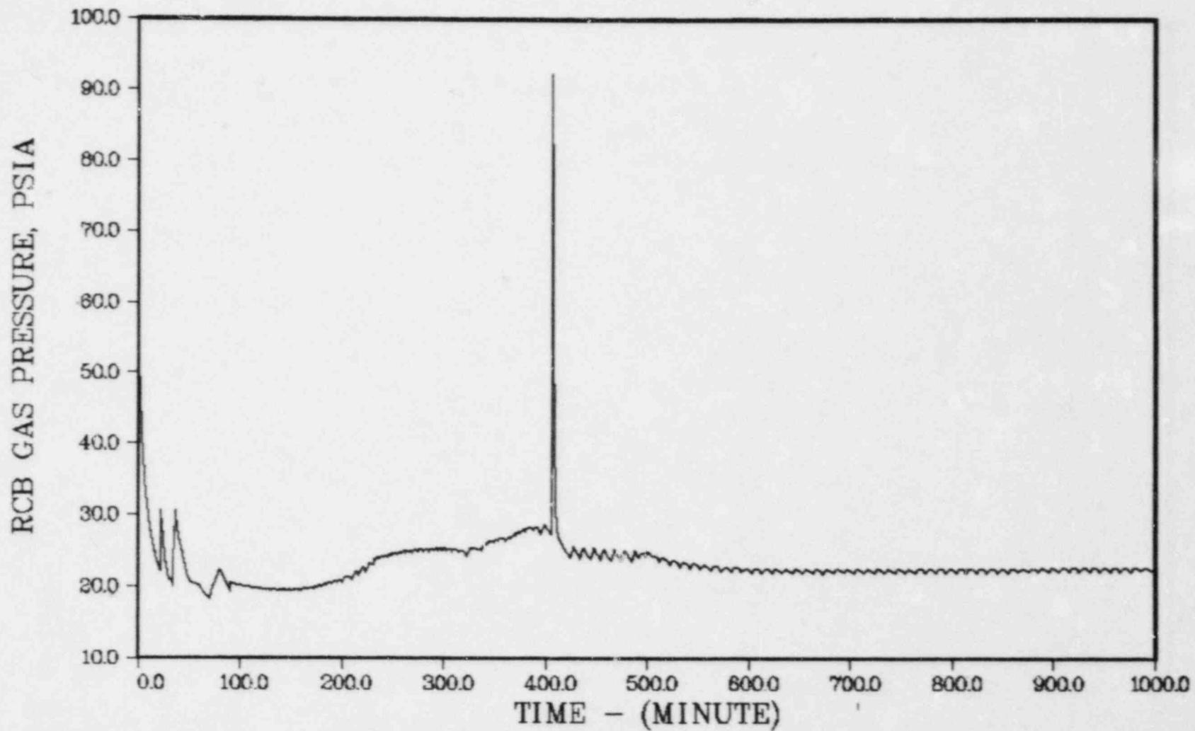
Figure 4.3-2. Zion AD (Double-Ended Cold-Leg Break) Containment Pressure Versus Time, MARCH 1.1 Calculation
