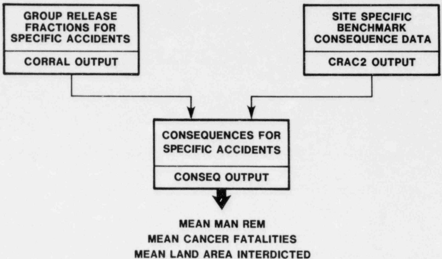
Figure 5.1-1. Method for Calculating Consequences
