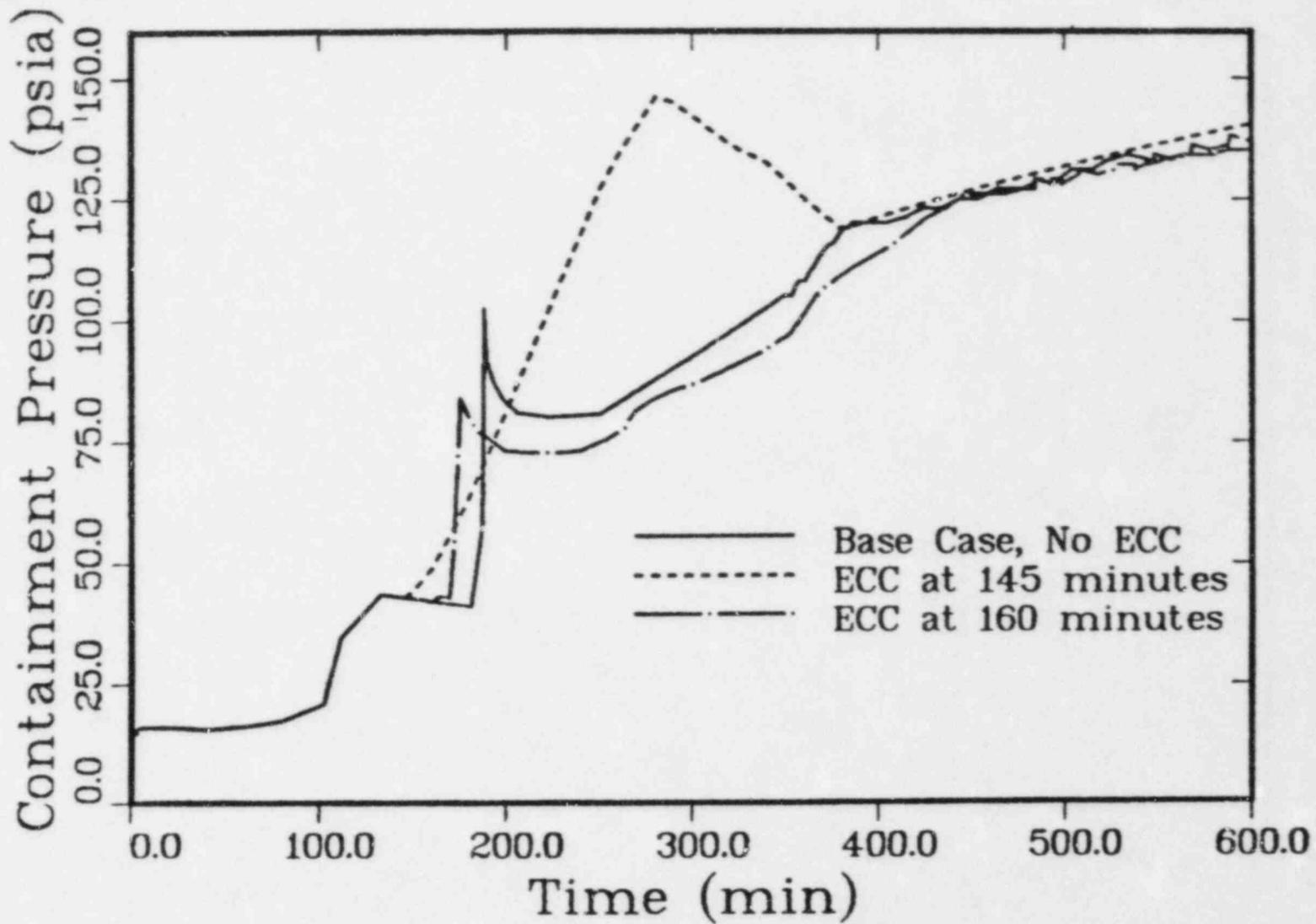
Figure 8.2-1. Zion TMLB' Containment Pressure Versus Time With Restoration of ECC but not Containment ESFs, MARCH 1.1 Calculations
