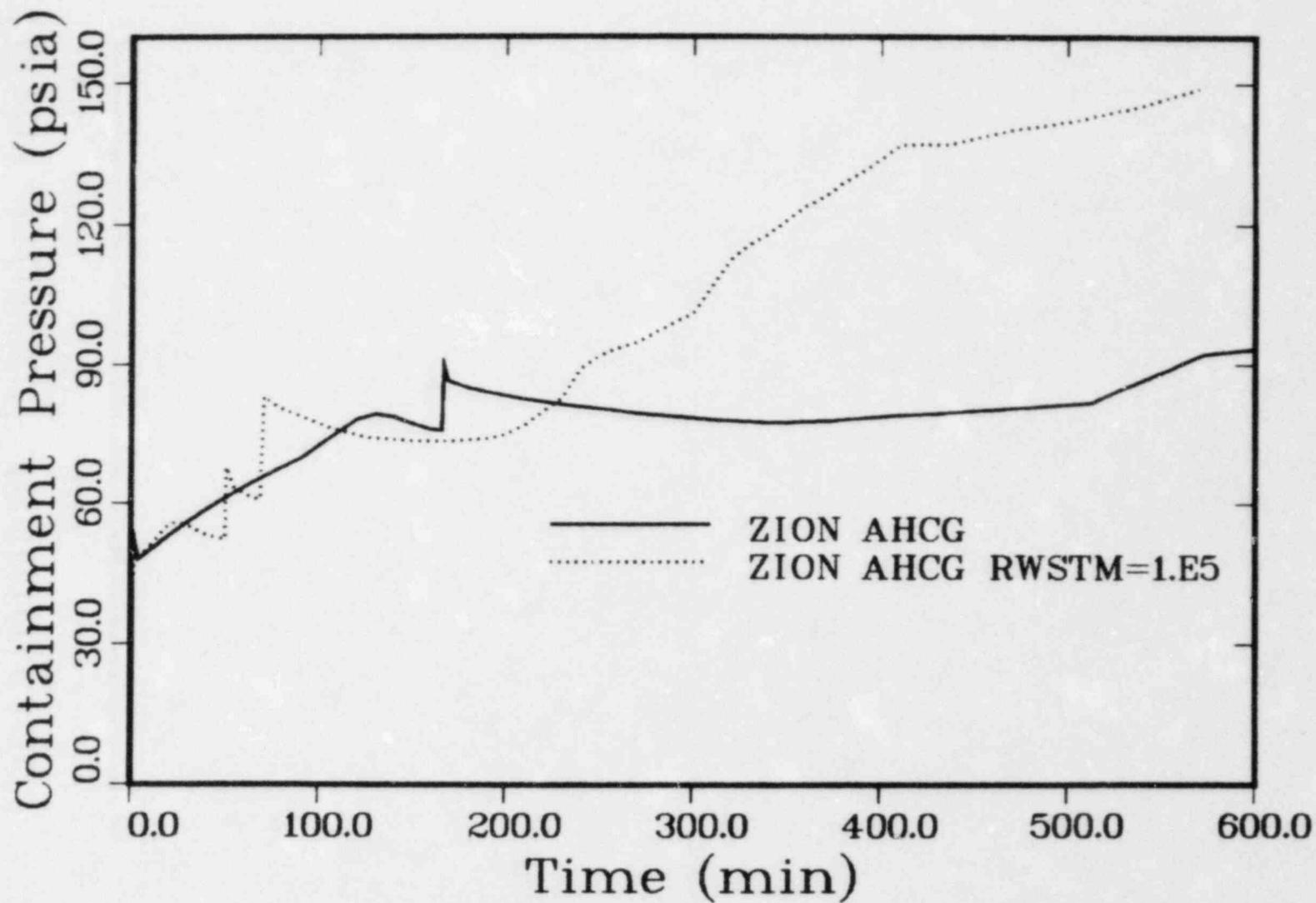
Figure 4.3-3. Zion AHCG (Double-Ended Cold-Leg Break) Containment Pressure Versus Time, MARCH 1.1 Calculation
