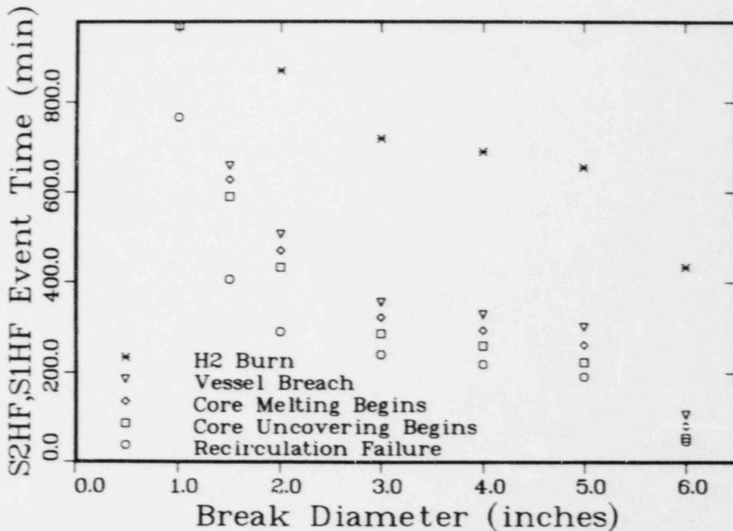
Figure 4.2.1-4. Zion S2HF and S1HF Accident Event Times Versus Break Size, MARCH 1.1 Calculations
