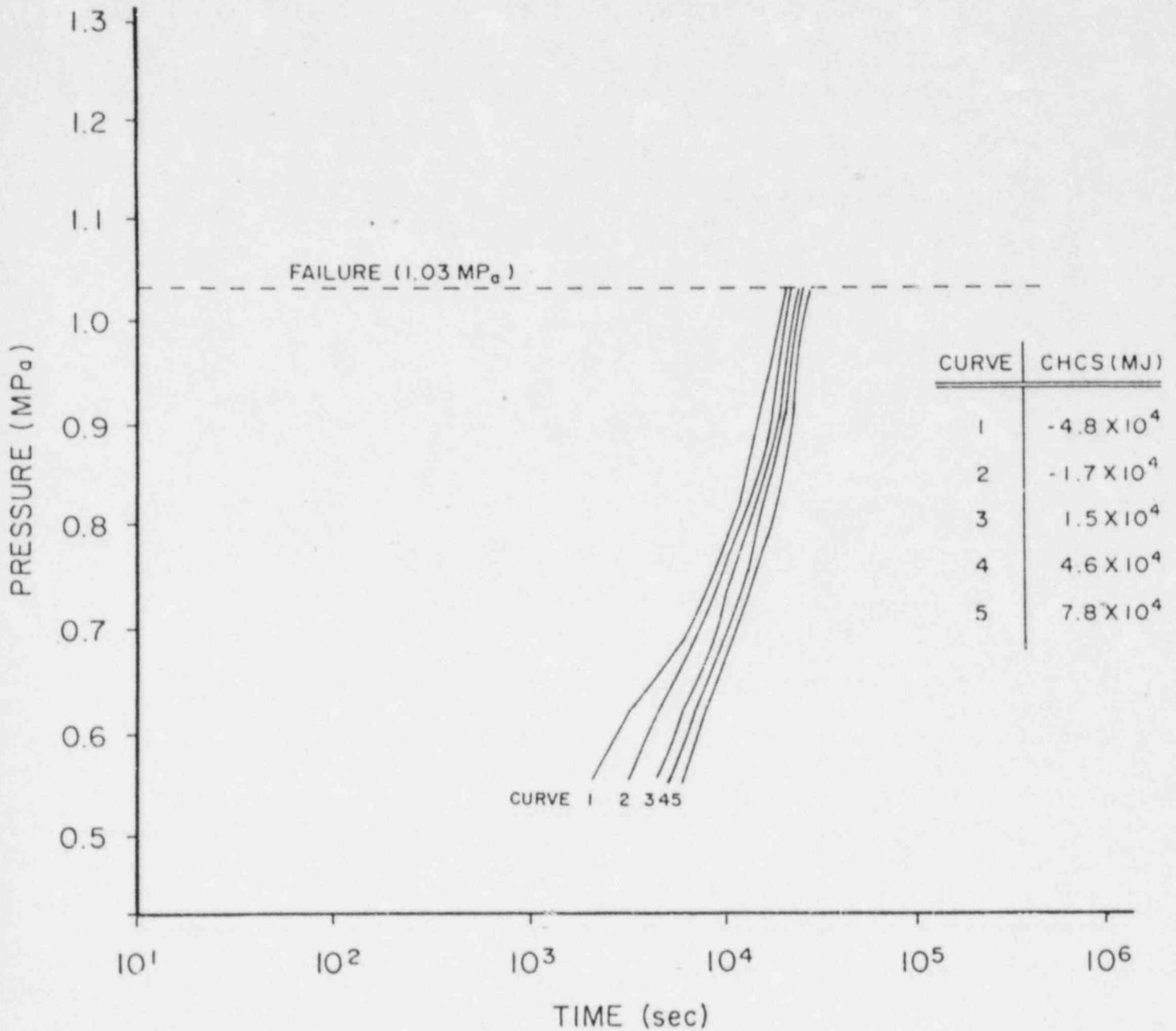
Figure C-1. Maximum Containment Pressurization When  $7 \times 10^4$  lb Water is Added.
