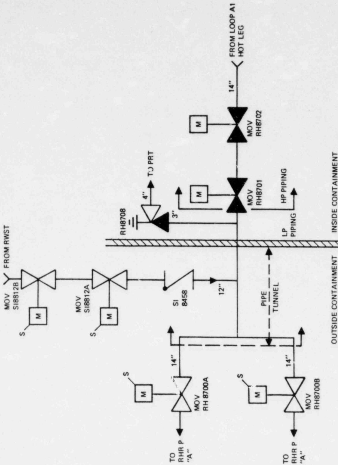
Figure 4.4-1. Schematic Diagram of Portion of RHR Suction Line Susceptible to V-Sequence Valve Failures
