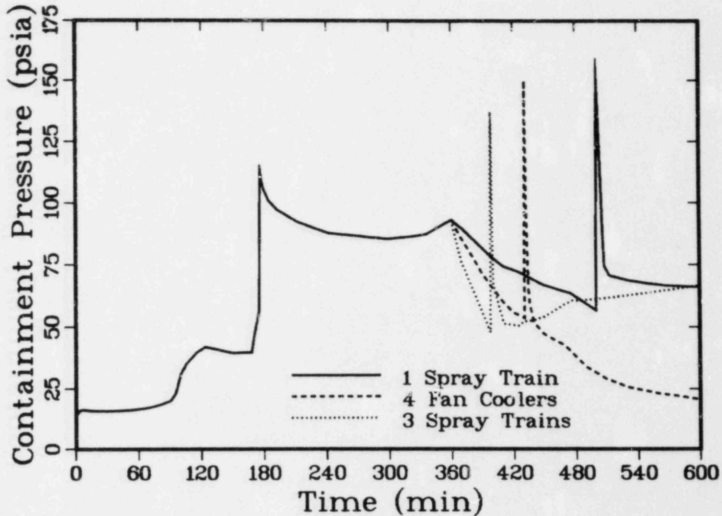
Figure 8.3.2-1. Zion TMLB' Containment Pressure Versus Time With Containment Cooling Restored After Vessel Breach, MARCH 1.1 Calculation
