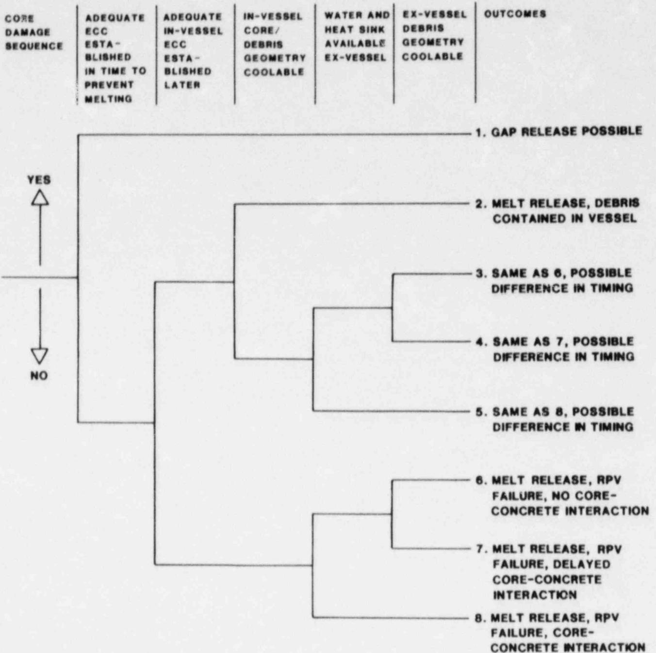
Figure 2-2. Core-Damage Event Tree
