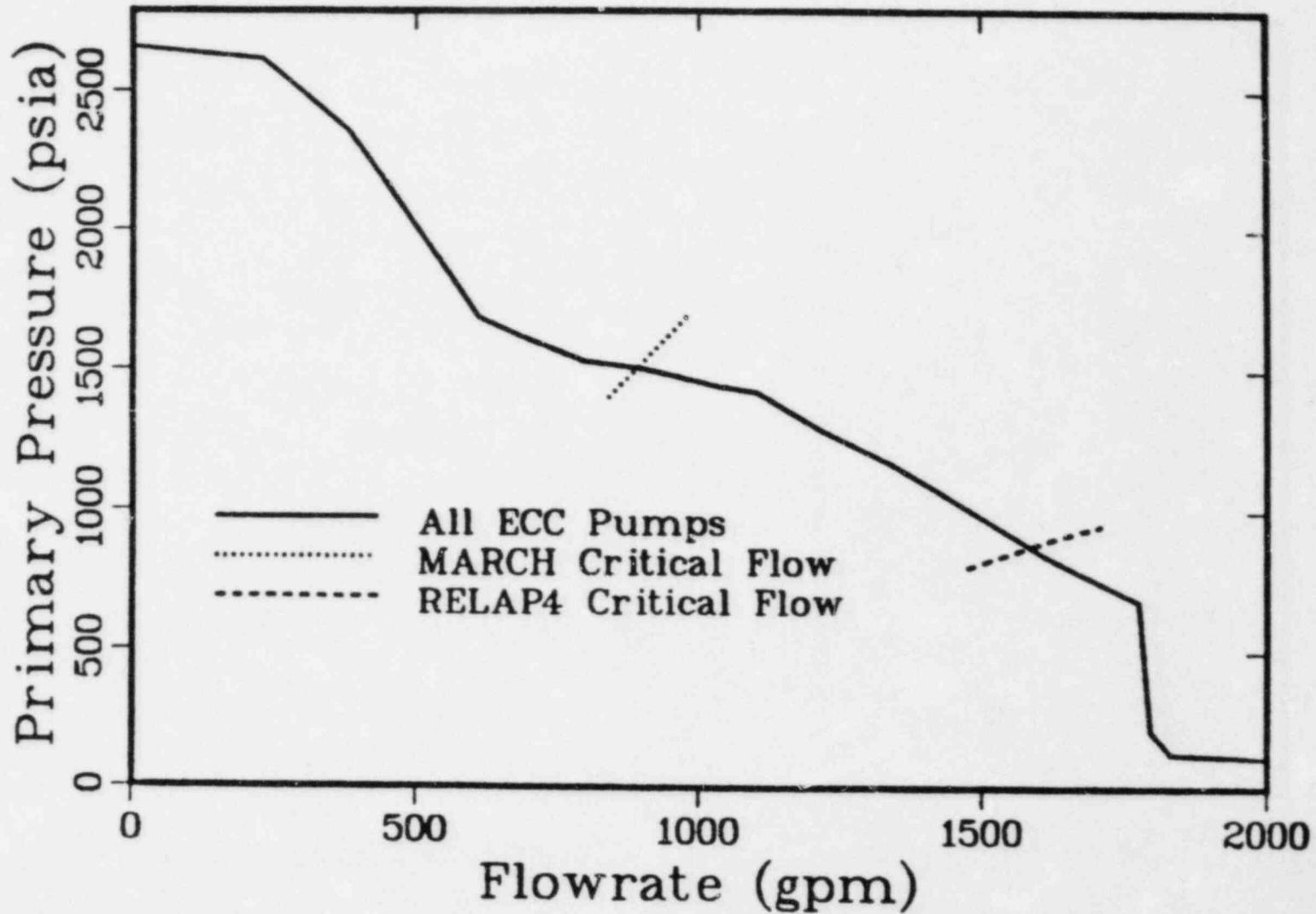
Figure 4.2.1-2. Pump Flow Curve Used for S2H Calculations Showing Differences Between MARCH and RELAP4 Critical Liquid Flows Through 1.5-Inch Diameter Break
