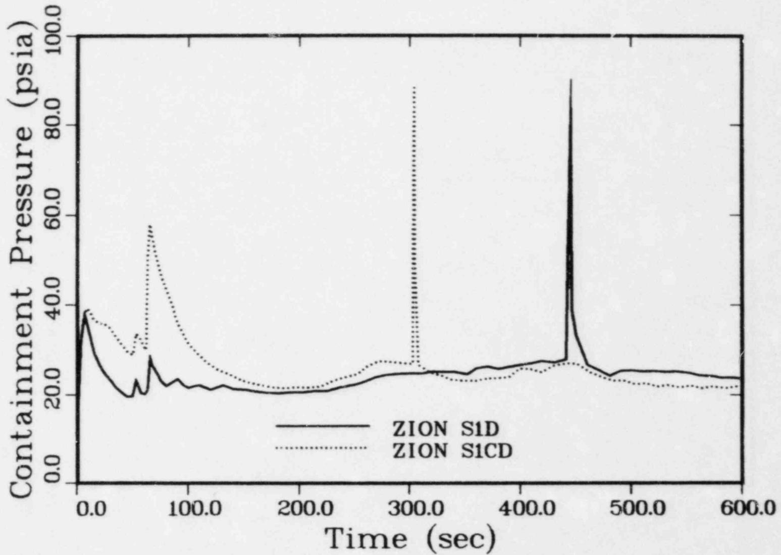
Figure 4.2.4-1. Zion S1D and S1CD (6 Inch Diameter Break)
