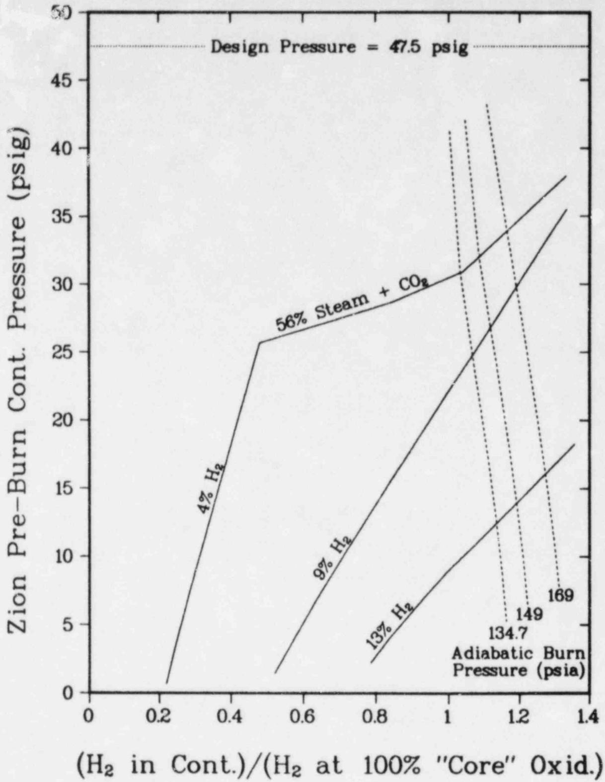
Figure 8.3-1. Containment Failure Estimates and Approximate Hydrogen Deflagration and Detonation Limits for the Zion Containment
