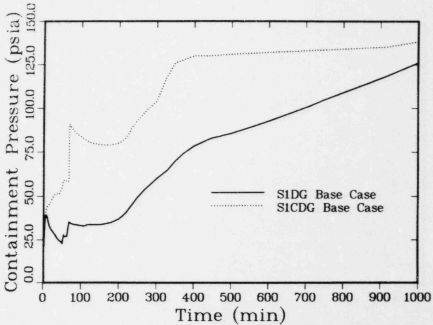
Figure 4.2.5-1. Zion S1DG and S1CDG (6-Inch Diameter Break)
