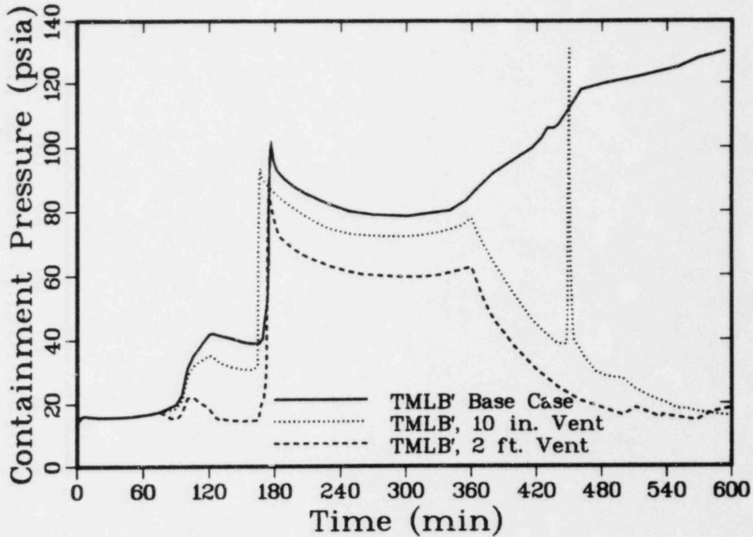
Figure 8.3.4-1. Zion TMLB' Containment Pressure Versus Time With Containment Venting Before Core Uncovering, MARCH 1.1 Calculation
