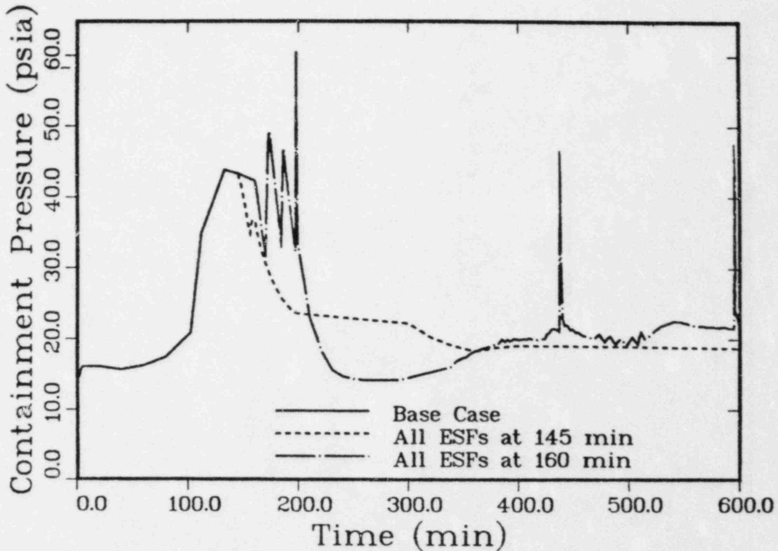
Figure 8.2-2. Zion TMLB' Containment Pressure Versus Time With Restoration of ECC and Containment ESFs, MARCH 1.1 Calculations
