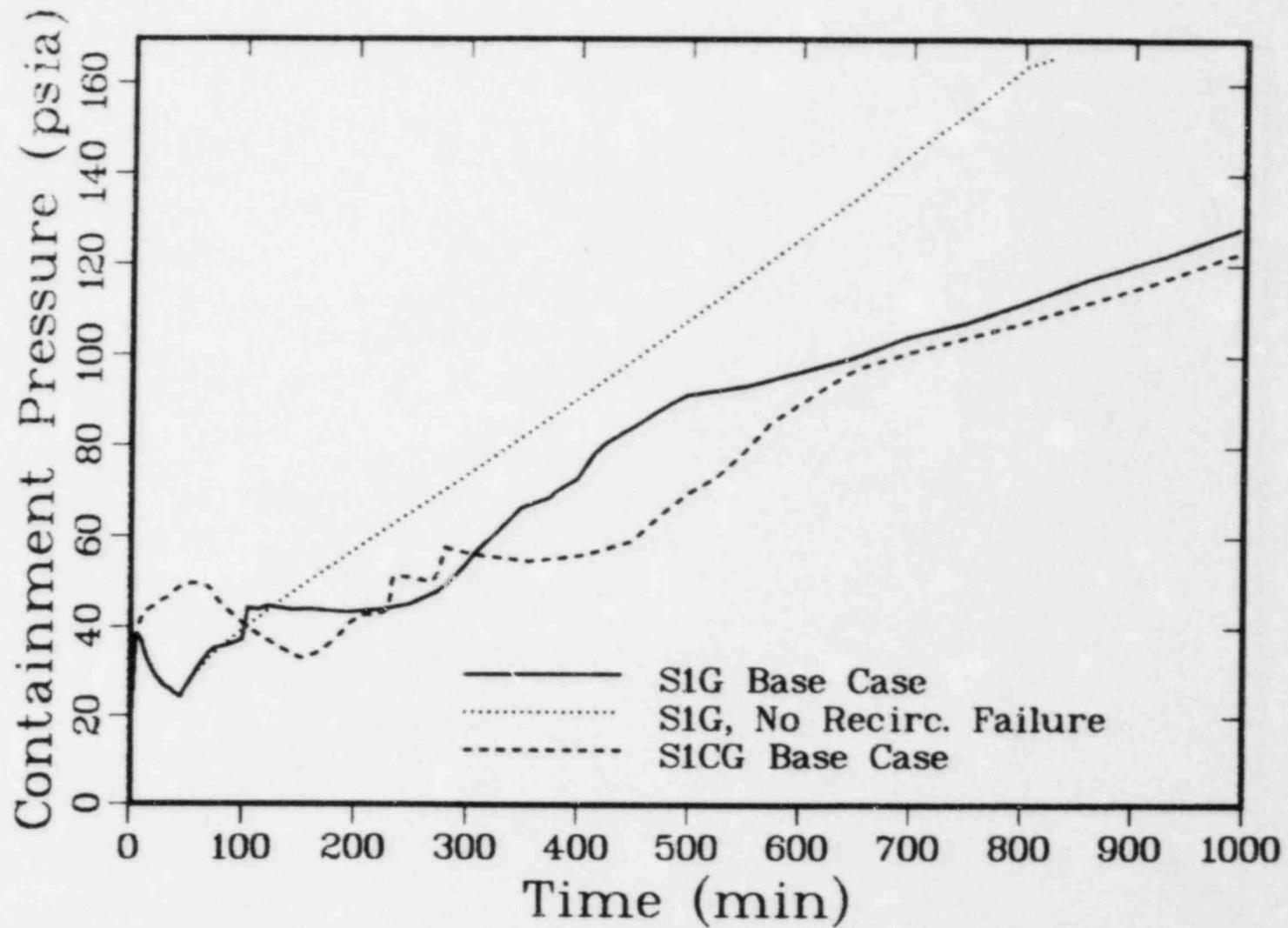
Figure 4.2.3-1. Zion S1G and S1CG (6-Inch Diameter Break) Containment Pressure Responses, MARCH 1.1 Calculations
