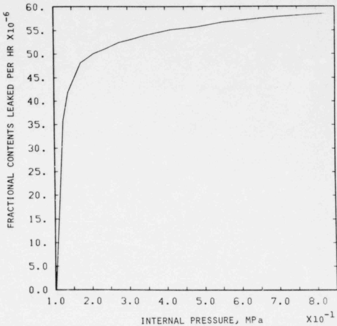
Figure 5.2-1. Containment Leakage as a Function of Internal Pressure
