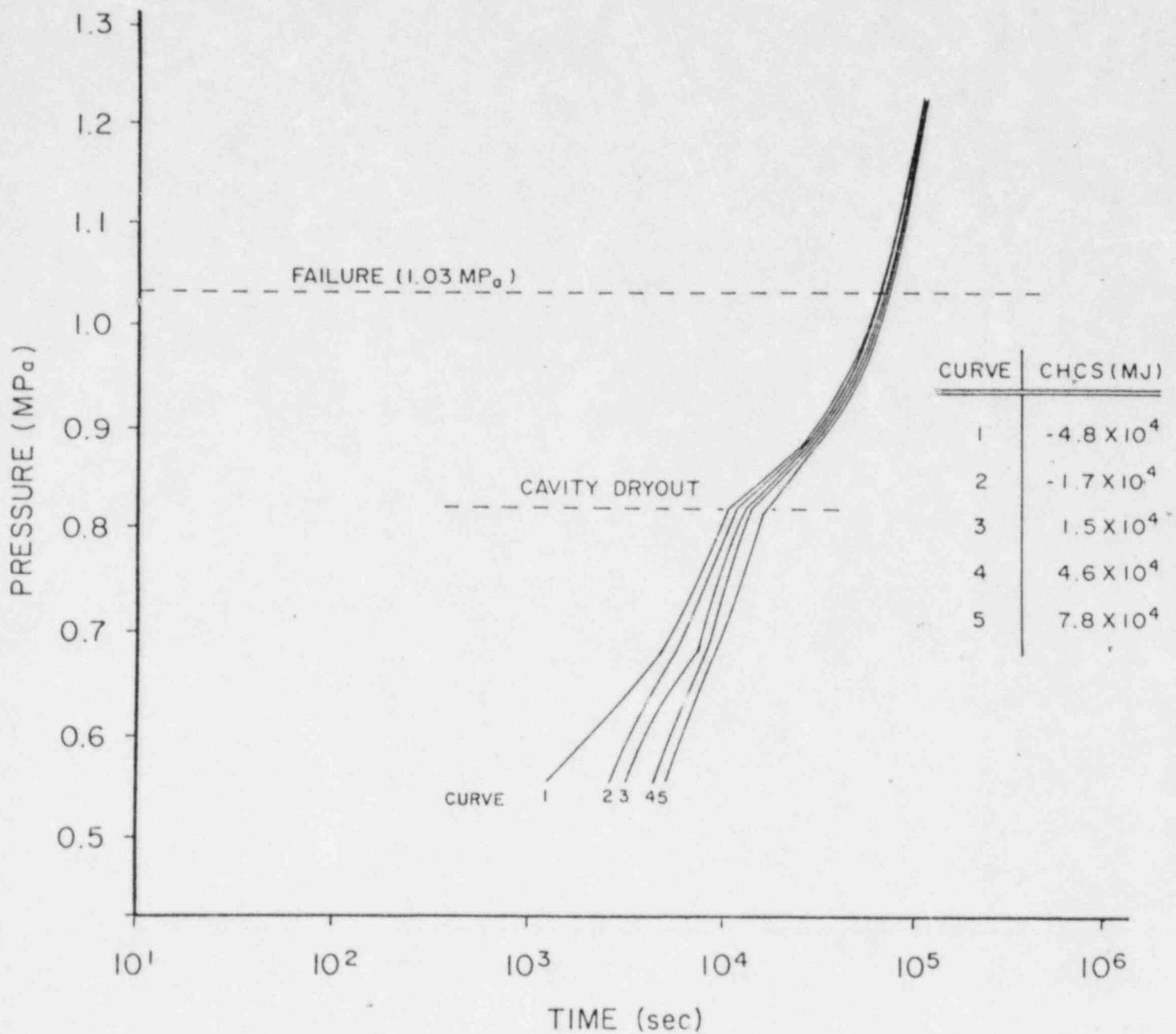
Figure C-3. Maximum Containment Pressurization When no Water is Added.
