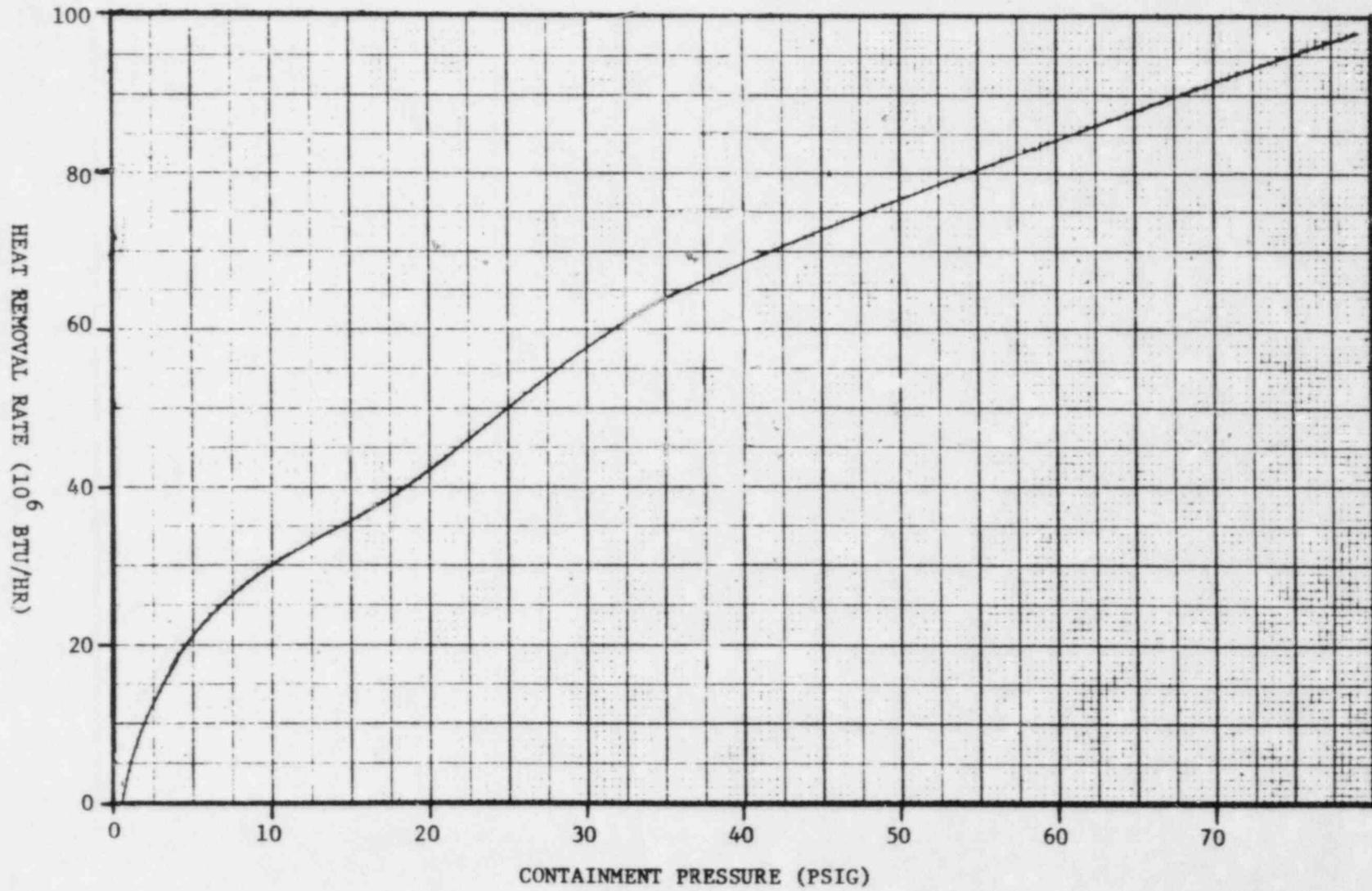
Figure C-4. Zion Fan Cooler Heat Removal Rate
