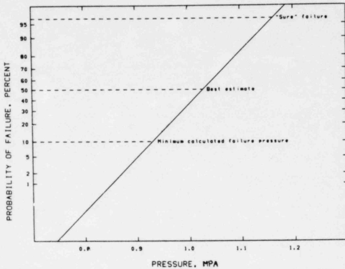
Figure B-1. Assumed containment failure probability distribution.
