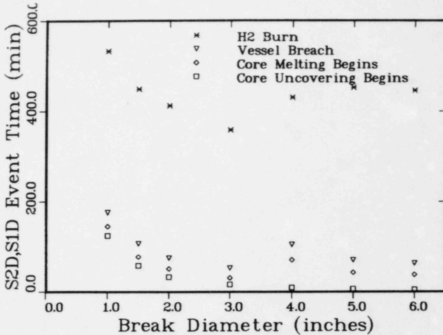
Figure 4.2.4-2. Zion S1D and S2D Accident Event Times Versus Break Diameter, MARCH 1.1 Calculations
