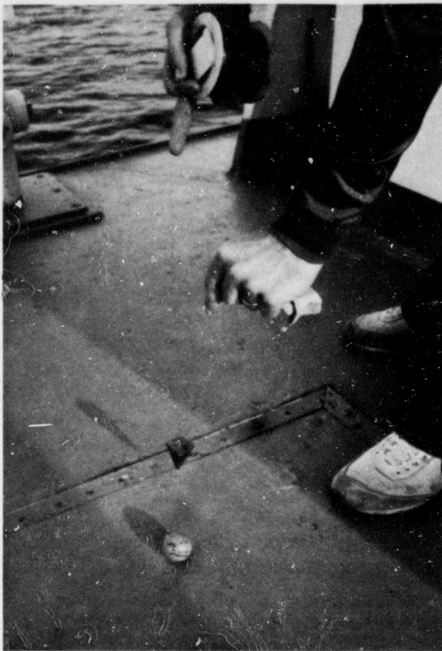
Fig. 37. The ping-pong ball standard target. A ping-pong ball, attached by monofilament line to a lead weight, makes a convenient standard target of about -42 dB. when suspended below the vessel and transducer. It allows calibration of the hydroacoustic equipment, a function vital to the accurate interpretation of hydroacoustic data. Photo by P. Kanciruk.
