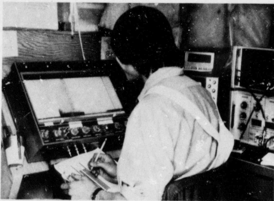
Fig. 23. Manual fish counting. Fish counts can be manually obtained from well-calibrated echograms if densities are low enough to avoid multiple returns. This method is, however, time-consuming and subject to operator bias. Automated methods of fish counting (or echo integration) should be employed whenever practical. Source: BioSonics, Seattle, Wash., with permission.
