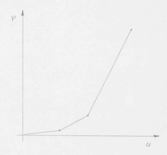
Typical stiffening force-displacement behavior for a nonlinear spring
