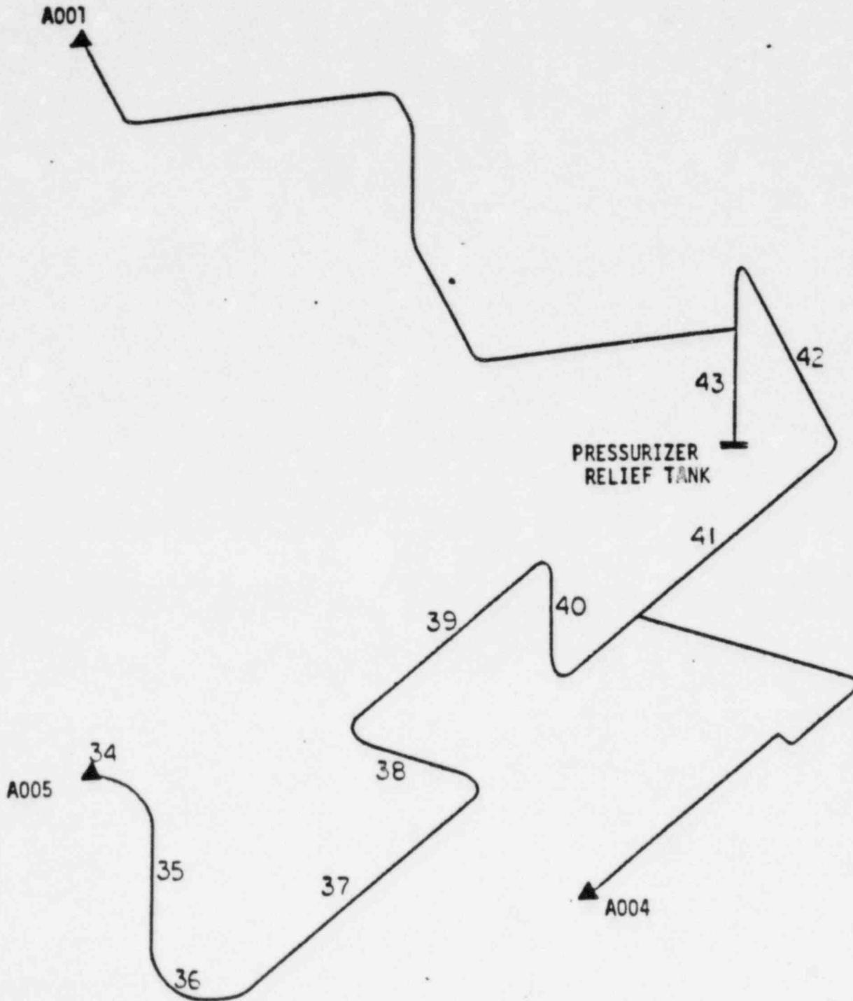
FIGURE 4-1B: SAFETY LINE HYDRAULIC MODEL
