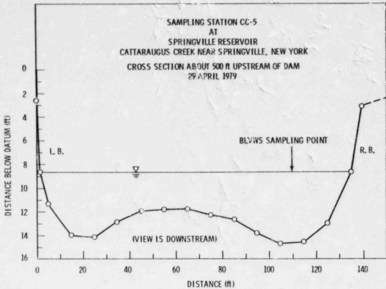
FIGURE A.21. Phase 3 Cross-Section at CC-5
