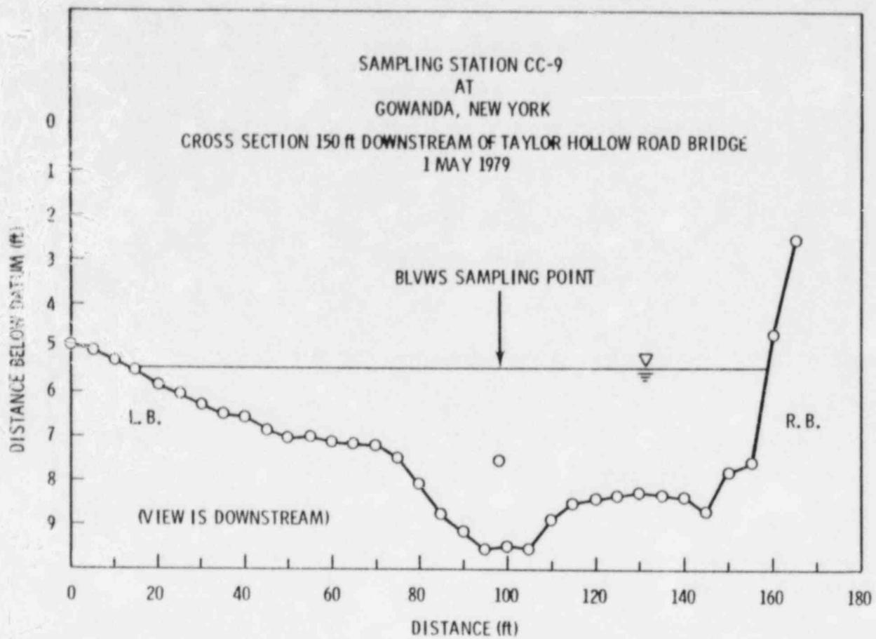
FIGURE A.25. Phase 3 Cross-Section at CC-9
