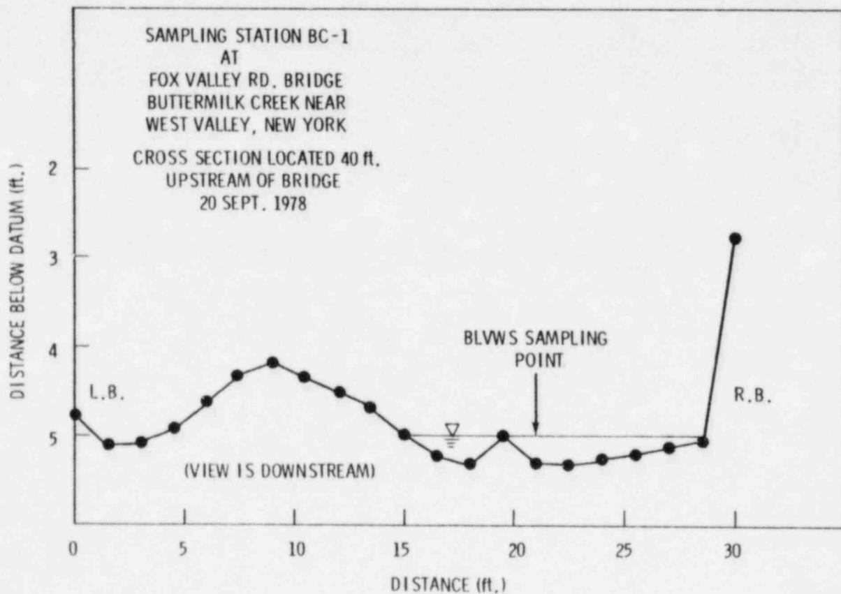
FIGURE A.5 Phase 2 Cross-Section at BC-1
