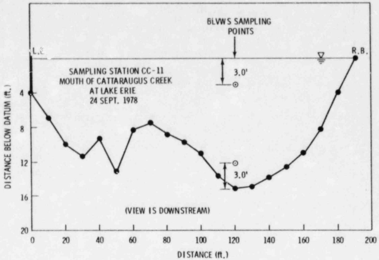
FIGURE A.27. Phase 2 Cross-Section at CC-11
