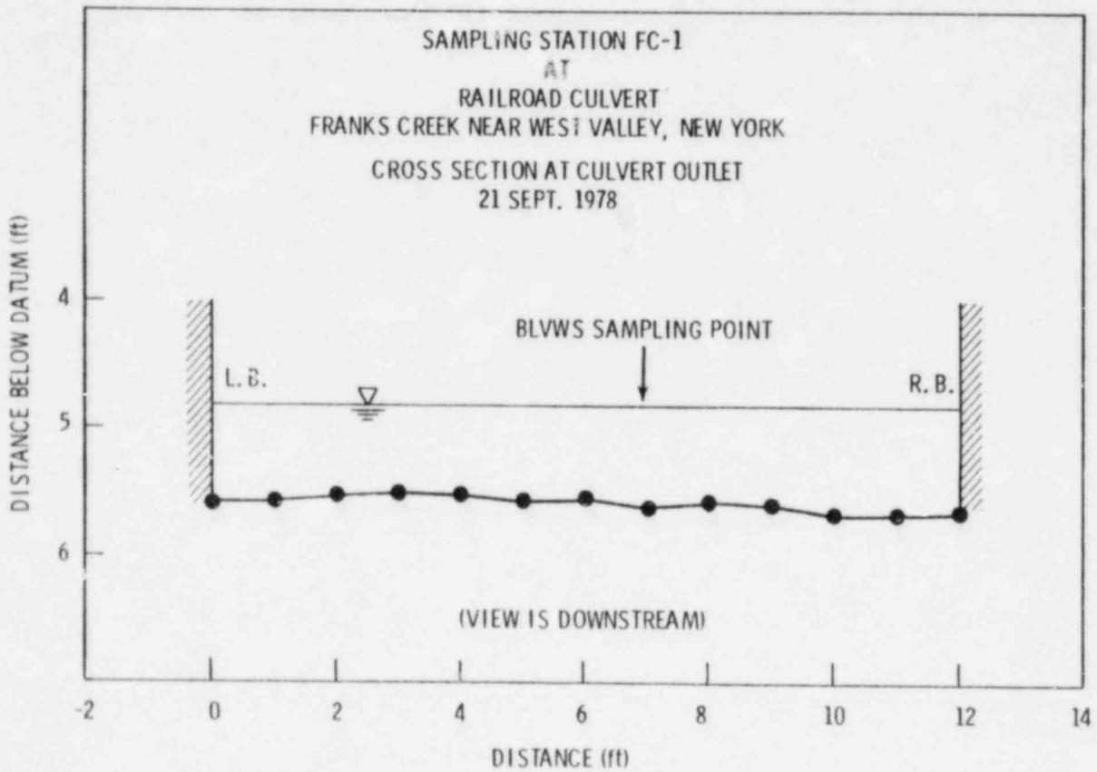
FIGURE A.2. Phase 2 Cross-Section at FC-1
