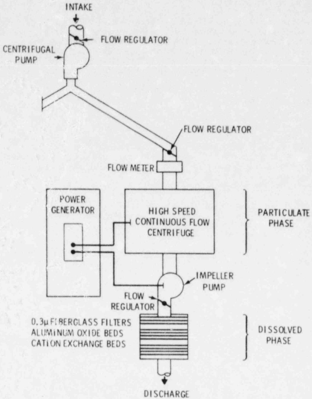
FIGURE 4. Phase 2 and 3 Sampling Apparatus
