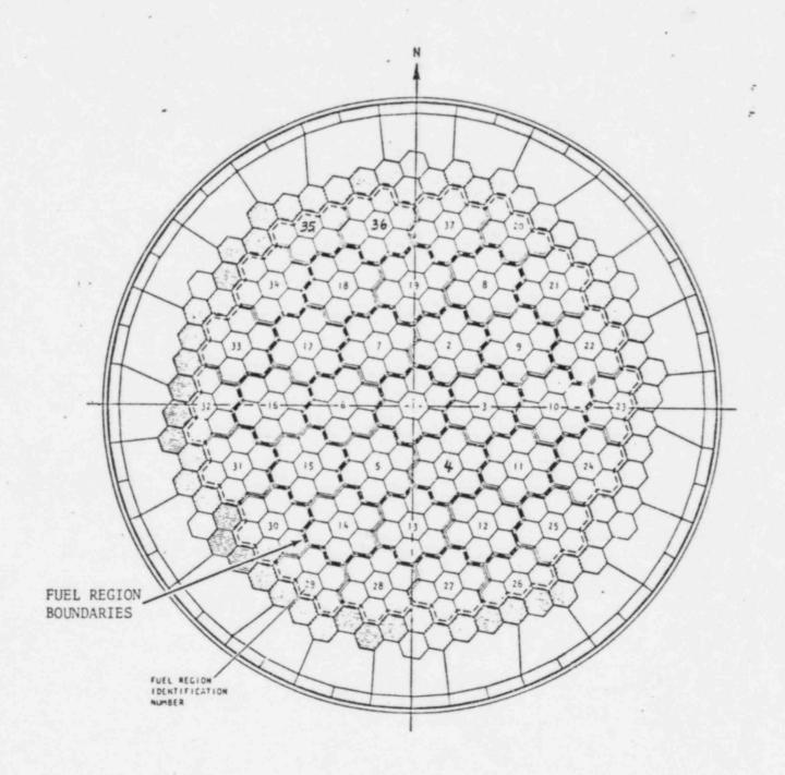
Fig. 3. Plan view of Fort St. Vrain reactor
