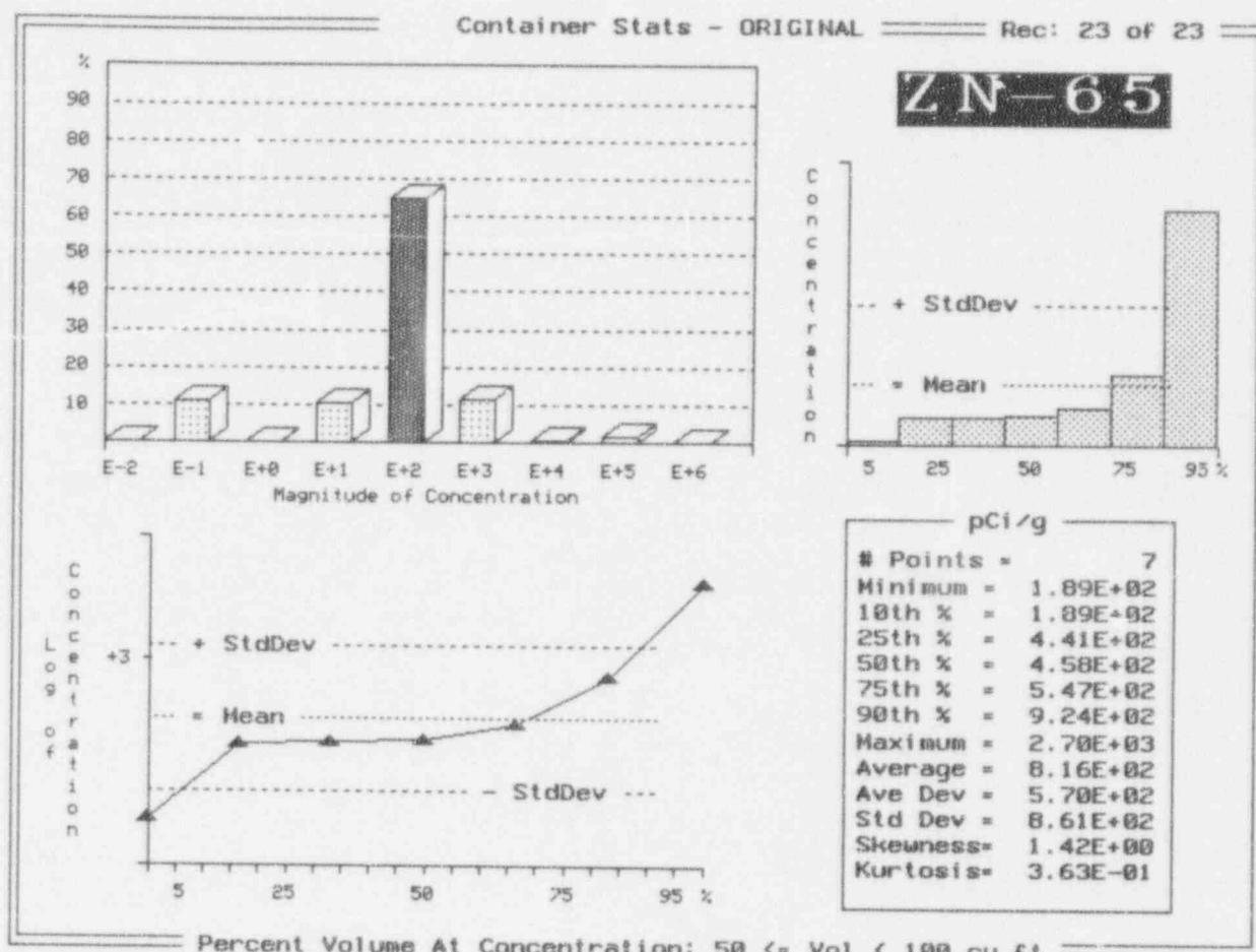
Exhibit K-2      Compacted Dry Active Waste Radionuclide
