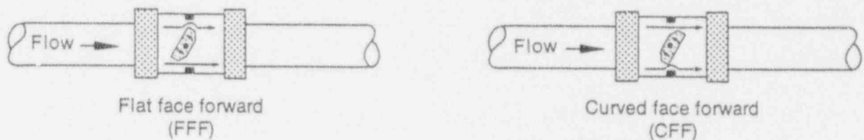
Figure 2-3. Valve orientations installed in the test section with uniform inlet flow.
