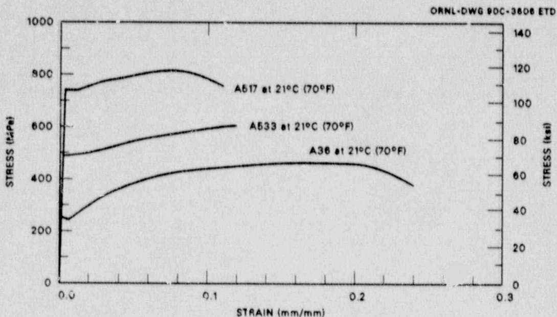
Fig. 13. Comparison of stress-strain curves for A36, A517, and A533 steels.
