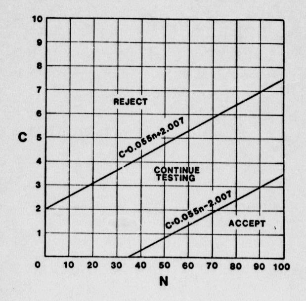
SAMPLE PLAN 2) FOR SNUBBER FUNCTIONAL TEST Figure 4.7.4-1
