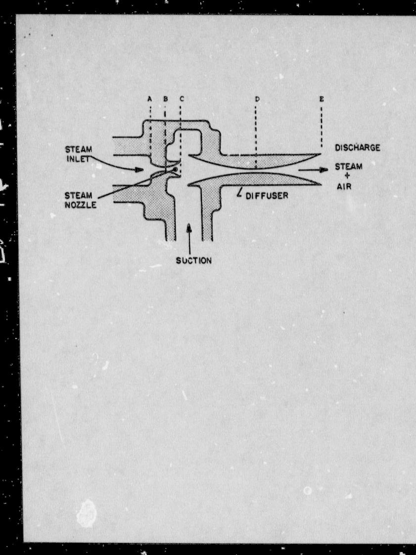
The plant is operating at 100 percent power when the only inservice steam jet air ejector is inadvertently isolated from the main condenser. The operator verifies circulating water system parameters have not changed. If no operator action is taken over the next 10 minutes, condenser vacuum will:
