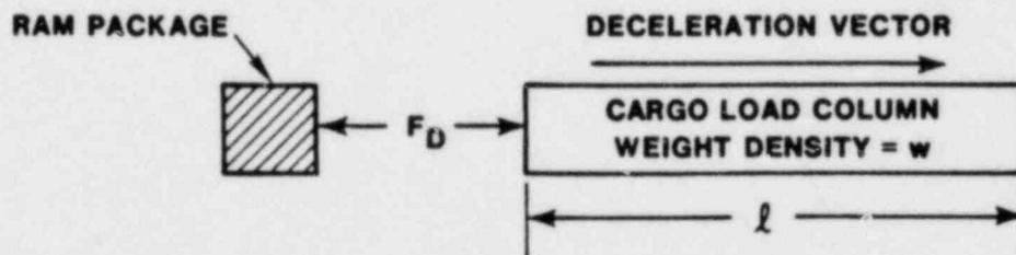
Figure 2. Free-Body Diagram--Cargo Load Column
