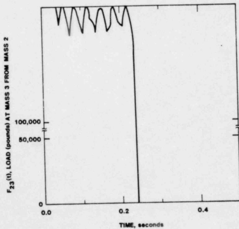
Figure 10. Dynamic Crush Load on RAM Package,  $F_{23}(t)$
