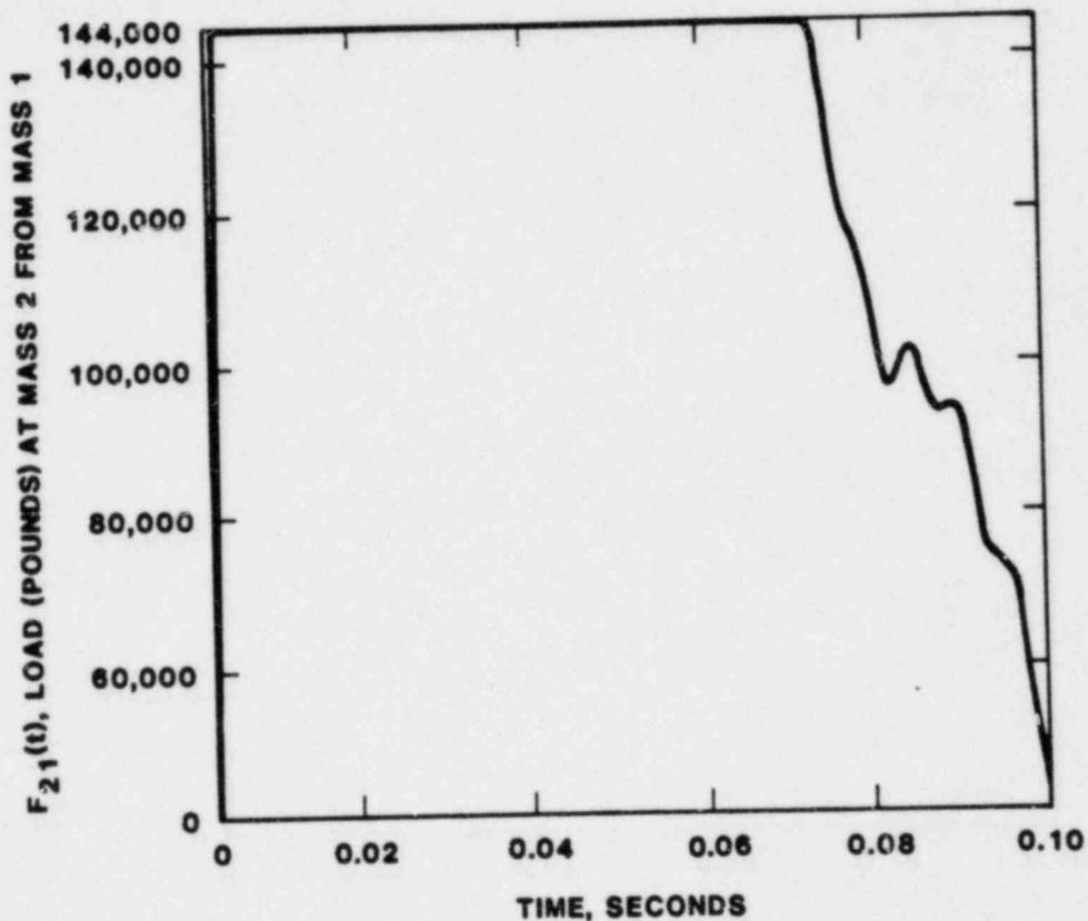
Figure 7. Dynamic Crush Load on RAM Package,  $F_{21}(t)$
