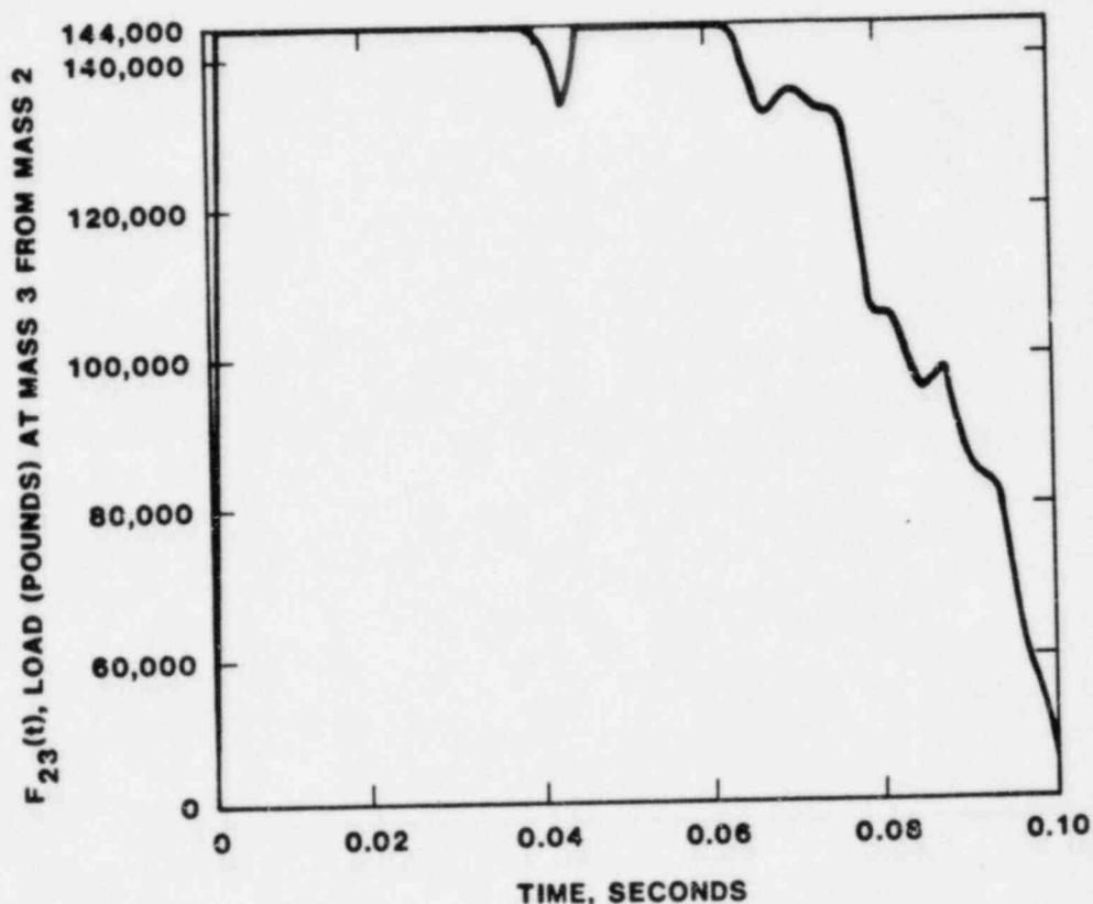
Figure 8. Dynamic Crush Load on RAM Package,  $F_{23}(t)$
