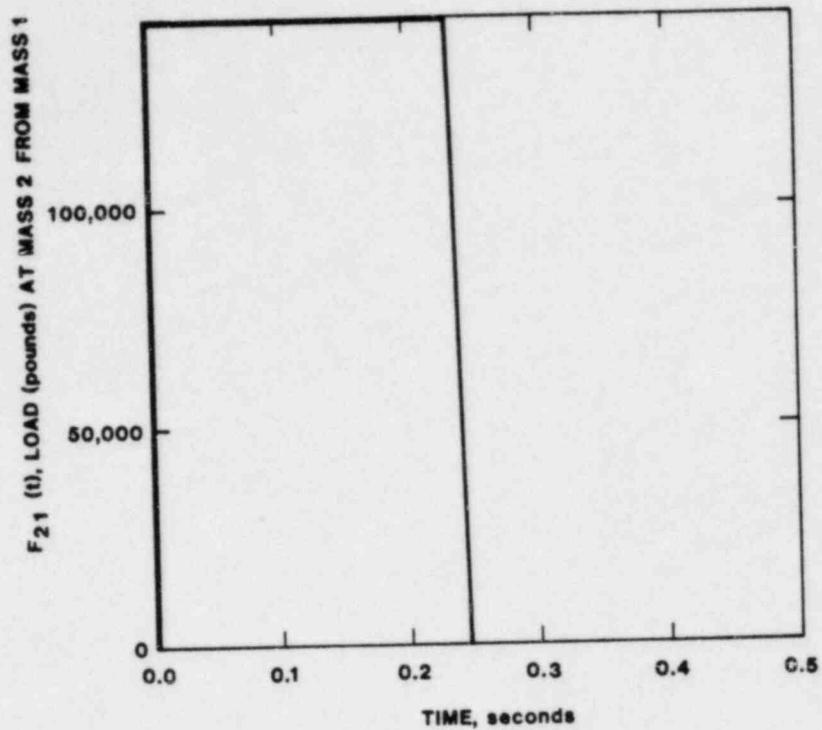
Figure 9. Dynamic Crush Load on RAM Package,  $F_{21}(t)$
