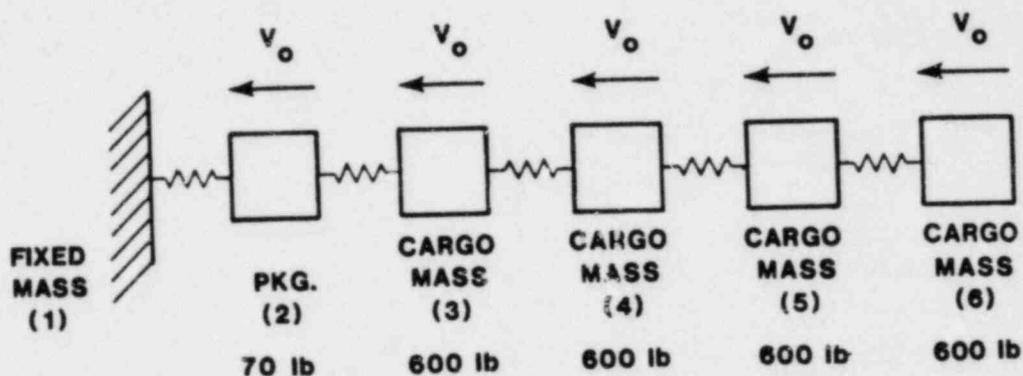
Figure 5. Lumped-Parameter Crush Model
