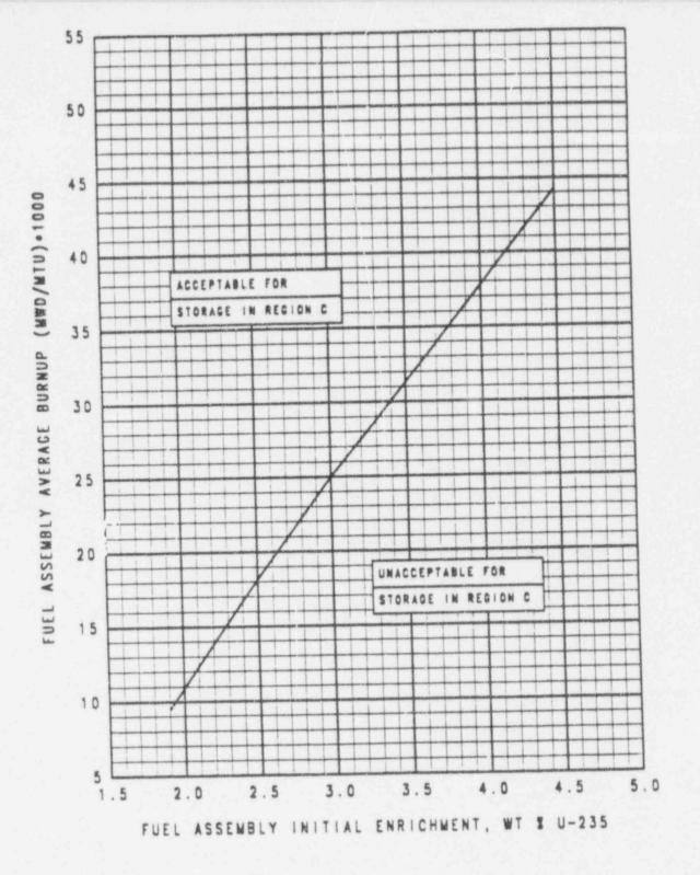
FIGURE 3.9-18 WINIMUM REQUIRED FUEL ASSEMBLY EXPOSURE AS A FUNCTION OF INITIAL ENRICHMENT TO PERMIT STORAGE IN REGION C WITH POISON PINS INSTALLED
