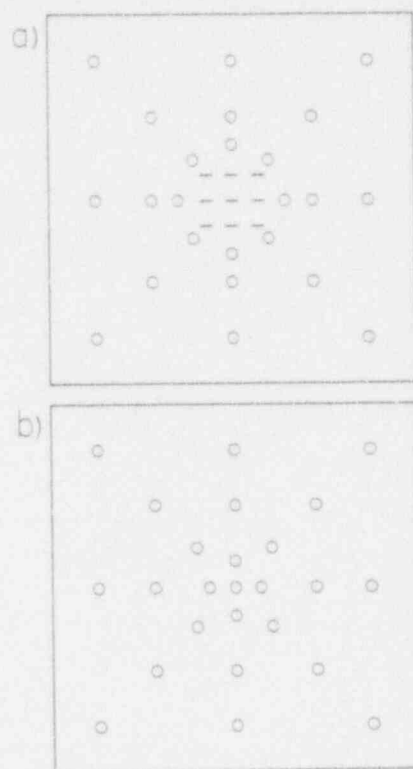
FIG. 1. TLD and source arrangement for multiseed two-plane implant experiment. The open circles are the position of TLD, carefully machined on slabs of Solid Water phantom. The phantom size is 20 \times 20 \times 20 \text{ cm}^3 .
