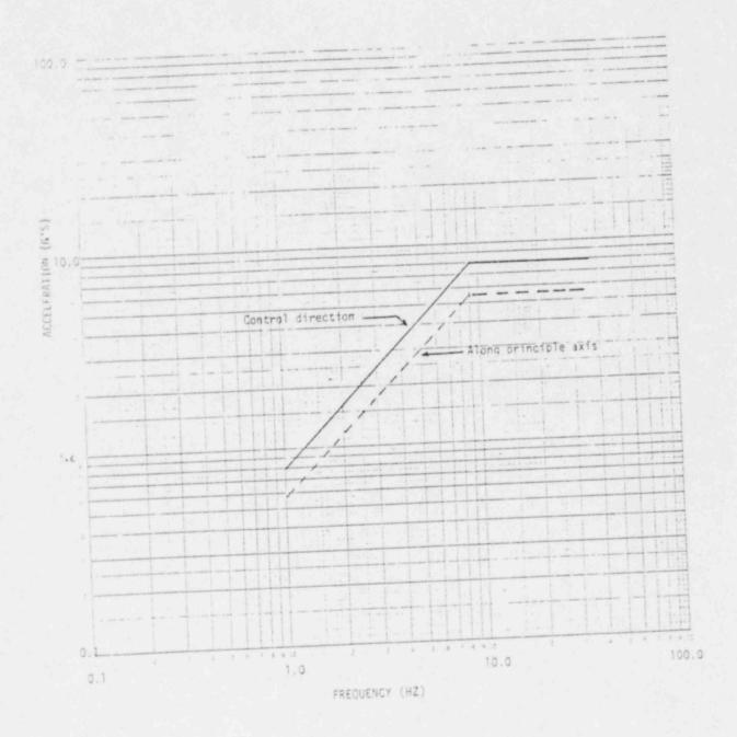
Figure 2. Safe Shutdown Earthquake Required Input Motion
