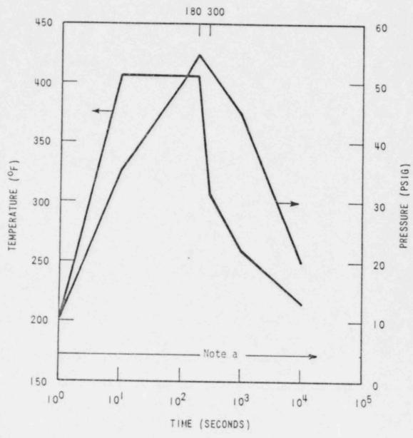
Note a: Initial 24 hour containment spray solution of 2500 ppm boron with 0.24% NaOH
