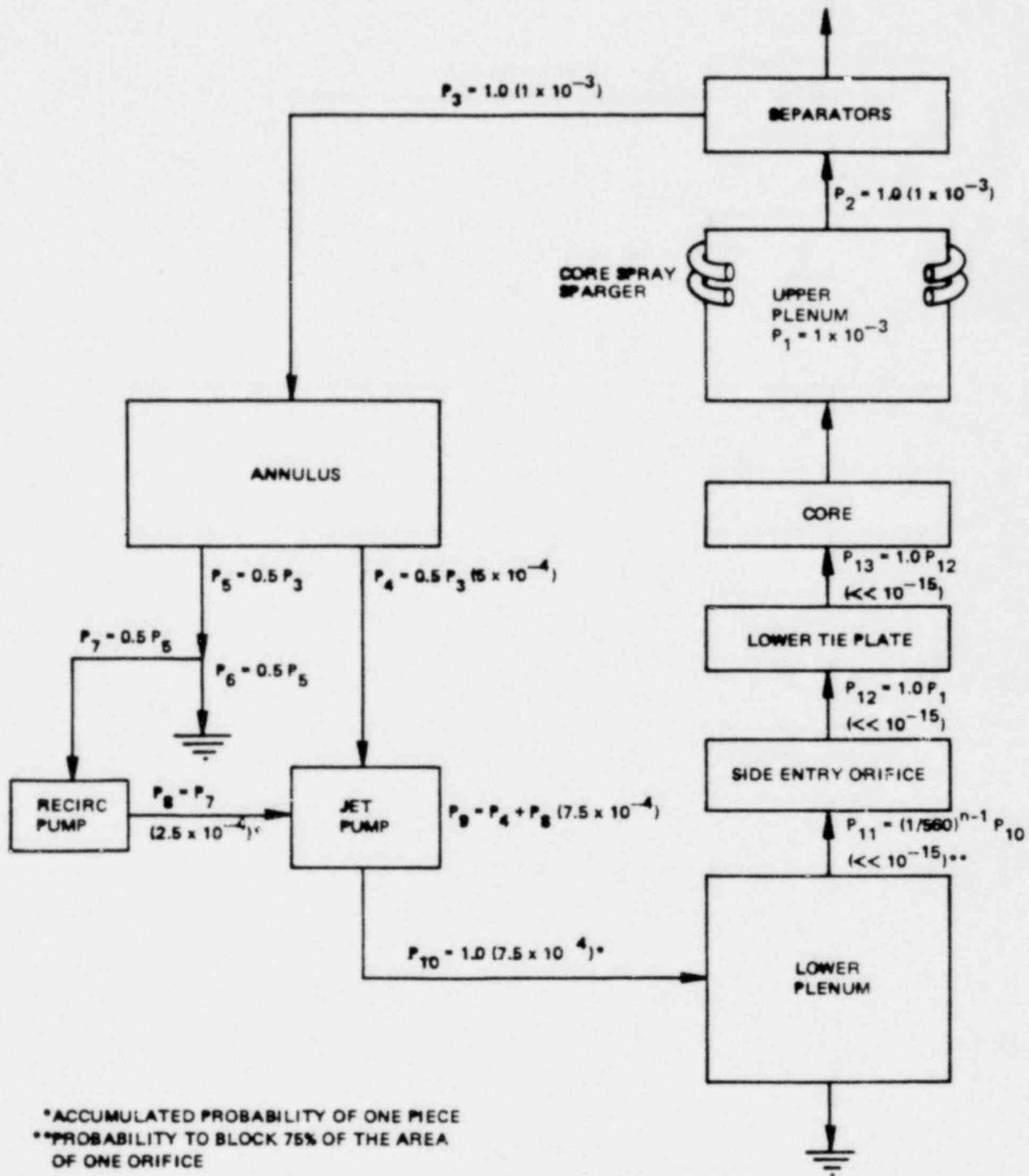
Figure 3-6. Loose Piece Potential Upward Flow Path
