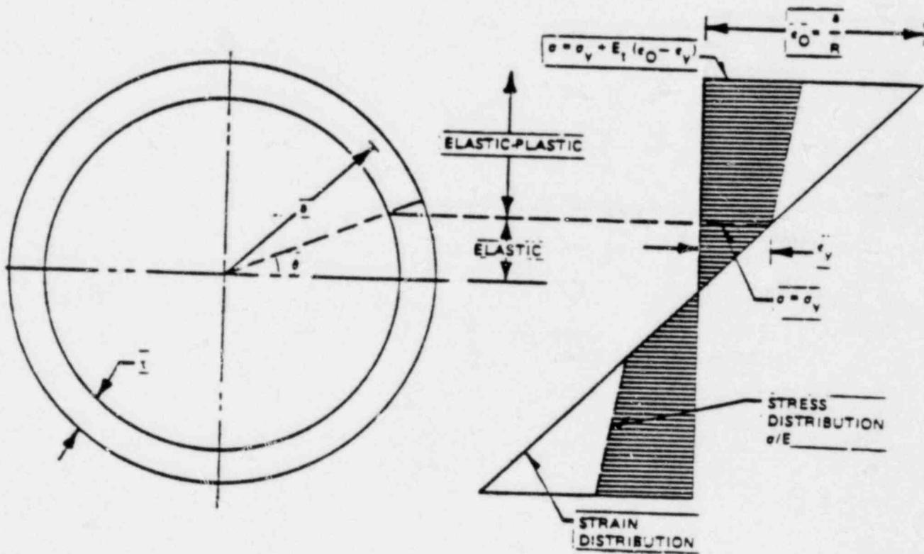
Figure 2-9. Stress and Strain Distribution in the Pipe Under Applied Moment
