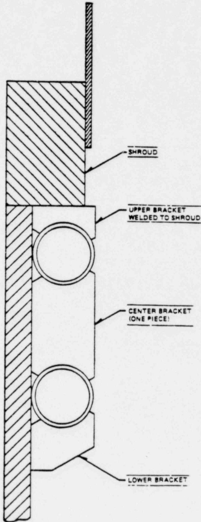
Figure 2-5. Sparger Support Method
