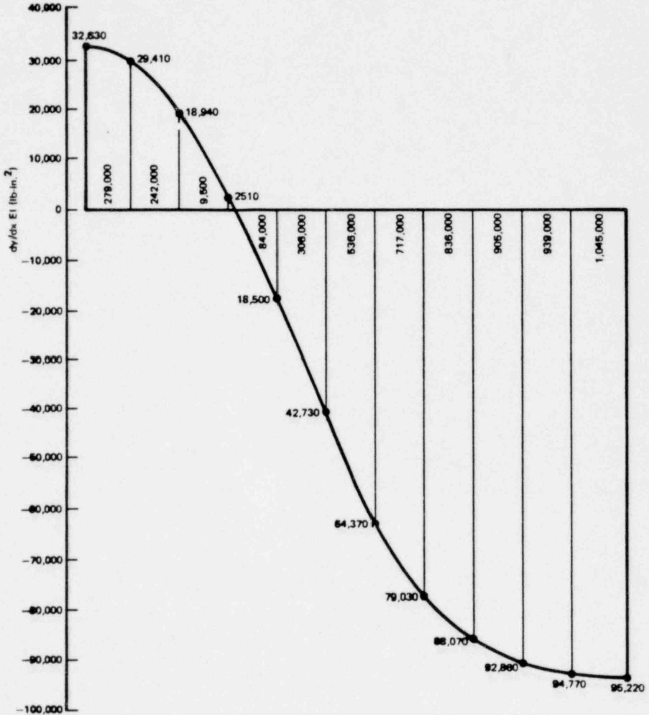
Graphical integration of the slope diagram yields deflections. The deflections must be adjusted so that the deflection at both brackets is zero.
