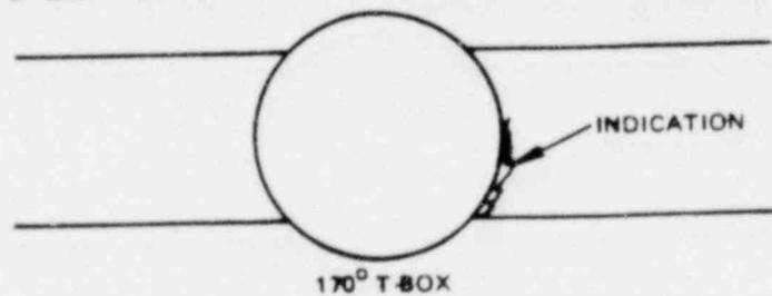
Figure 1-lb. Elevation View of Cracked Core Spray Sparger
