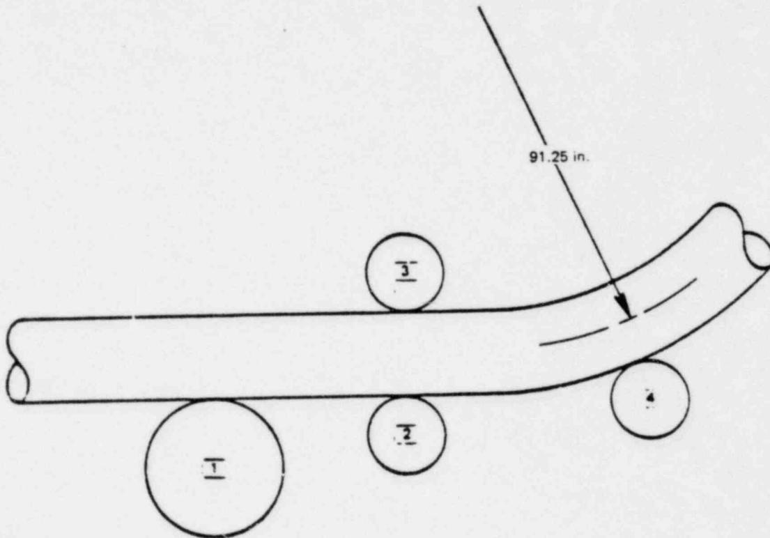
Figure 2-6. Pipe Bending Method
