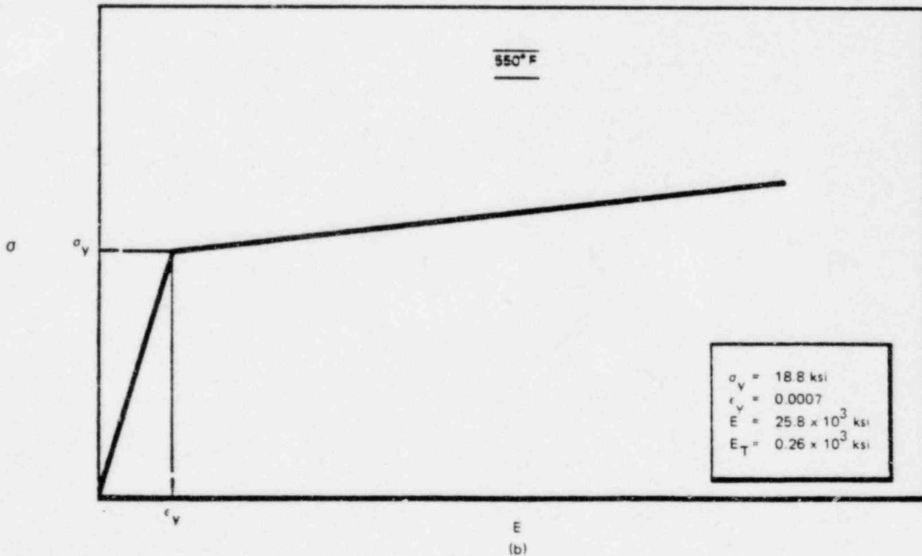
Figure 2-8. Bilinear Stress-Strain Curves for Type-304 Stainless Steel
