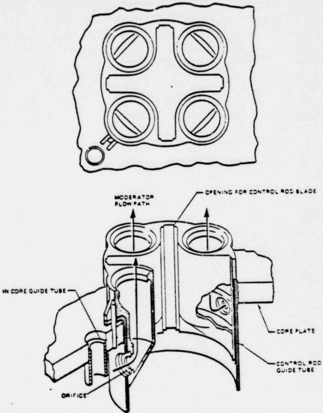
Figure 3-4. Orificed Fuel Support
