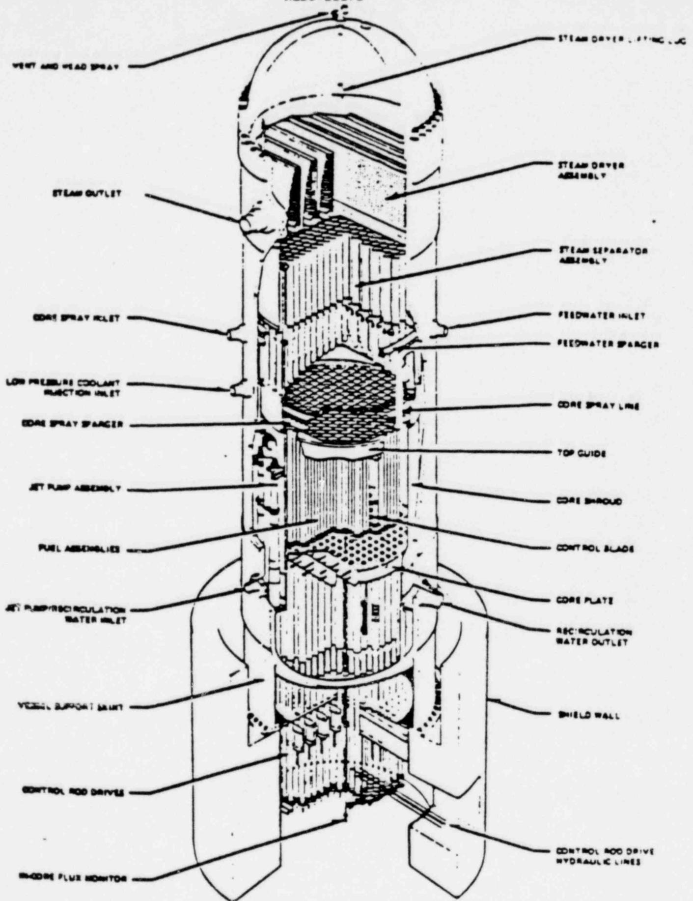
Figure 3-1. Reactor Vessel
