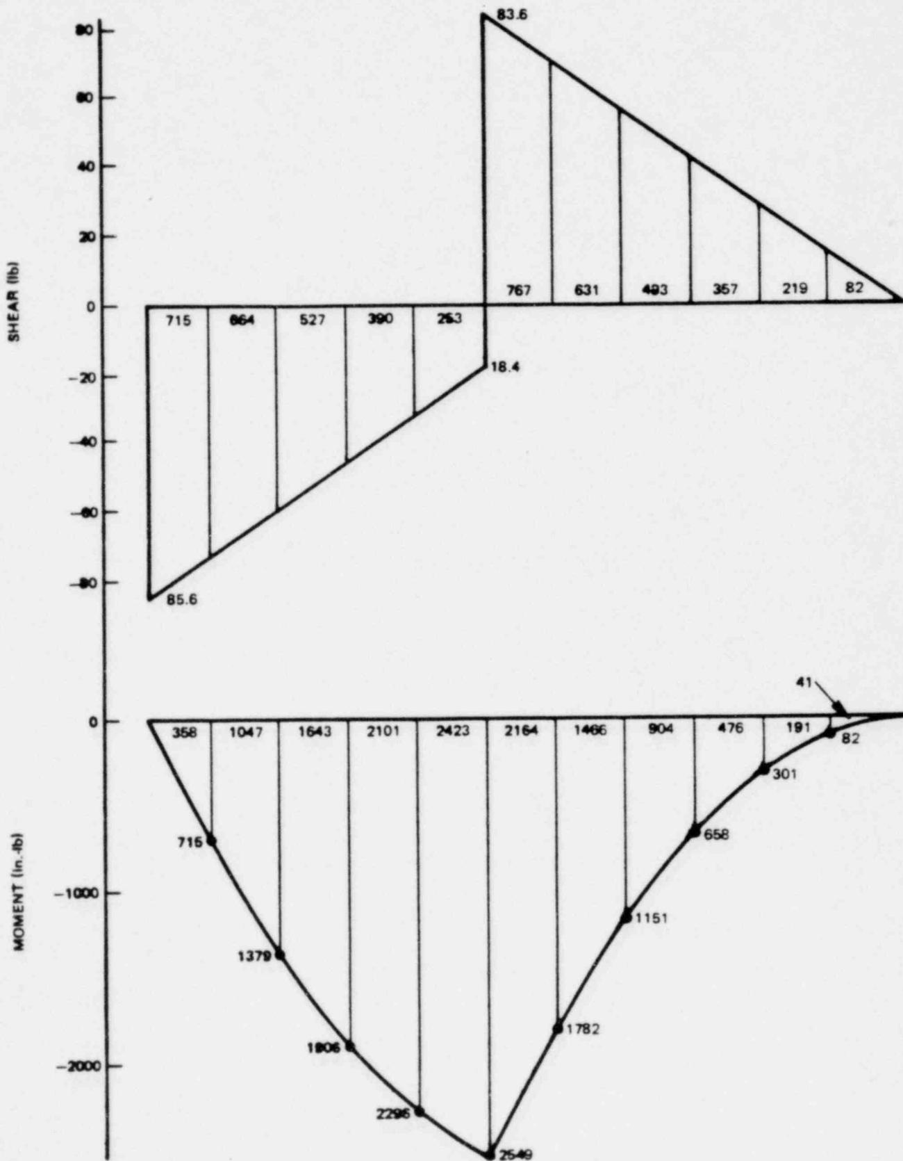
The slope ( $dy/dx$ ) diagram is now constructed by graphical integration of the moment diagram.
