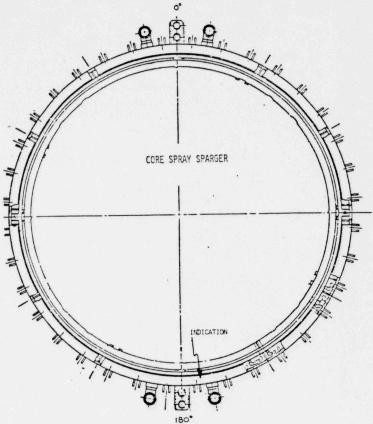
Figure 1-la. Plan View of Cracked Core Spray Sparger
