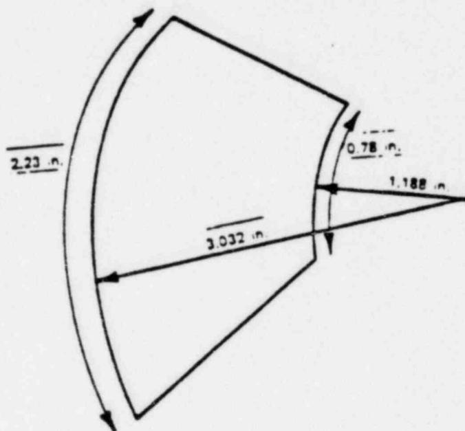
Figure 3-3. Largest Piece That Can Fit Through the Turning Vane (End View)
