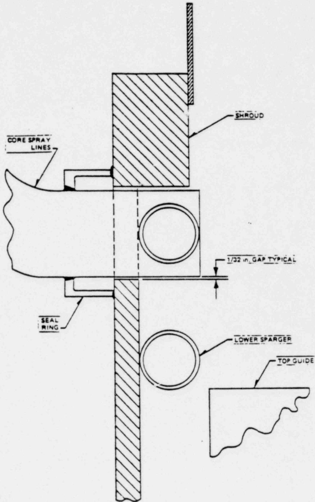
Figure 2-3. Sparger to Shroud Attachment Method
