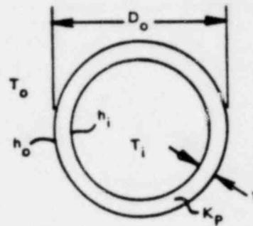
$$D_o = 4.0 \text{ in.} \quad t = 0.226 \text{ in.} \quad D_i = 3.548 \text{ in.}$$
