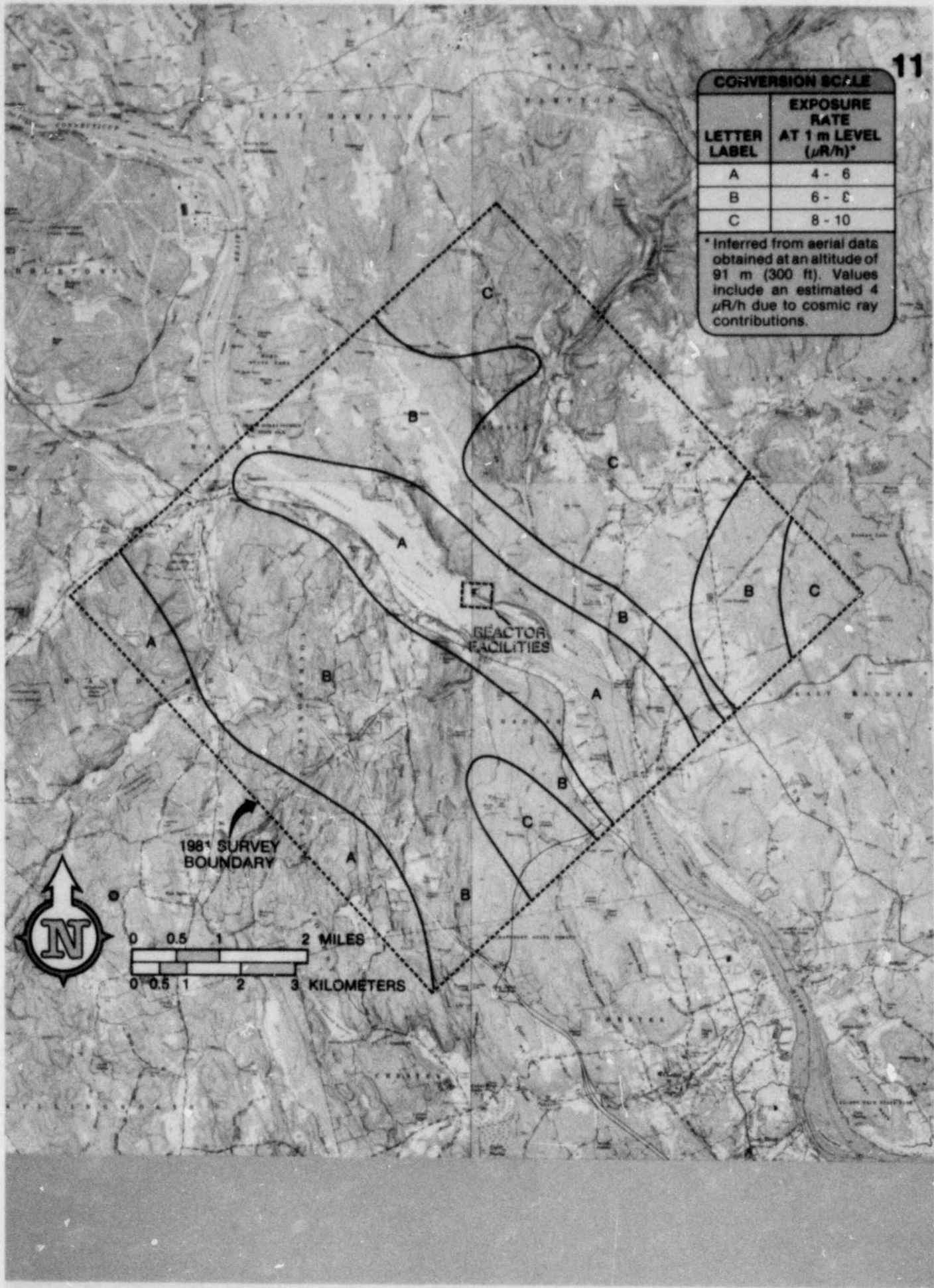
Figure 7. EXPOSURE RATE CONTOUR MAP SUPERIMPOSED ON USGS MAP OF THE AREA SURROUNDING THE HADDAM NECK PLANT (1969 SURVEY)
