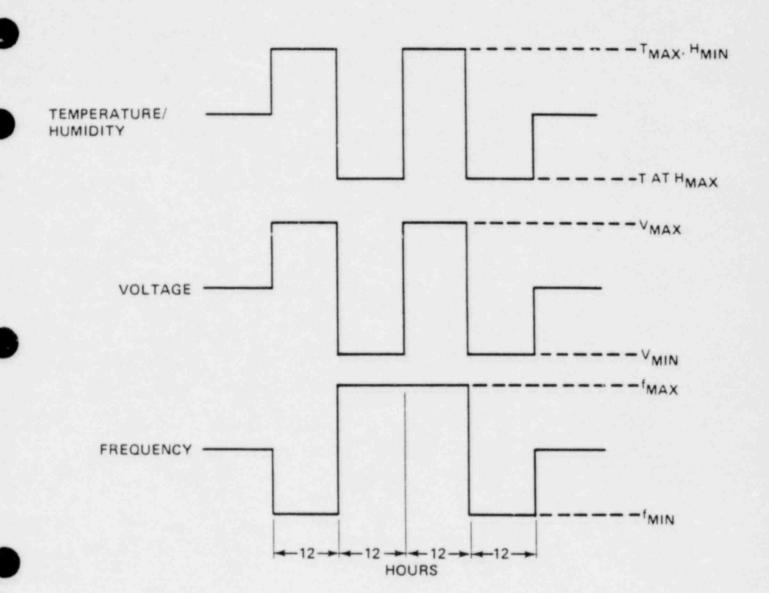
Figure 3 Verification Test Profile
