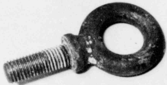
FIGURE 8 - Eyebolt after test.
