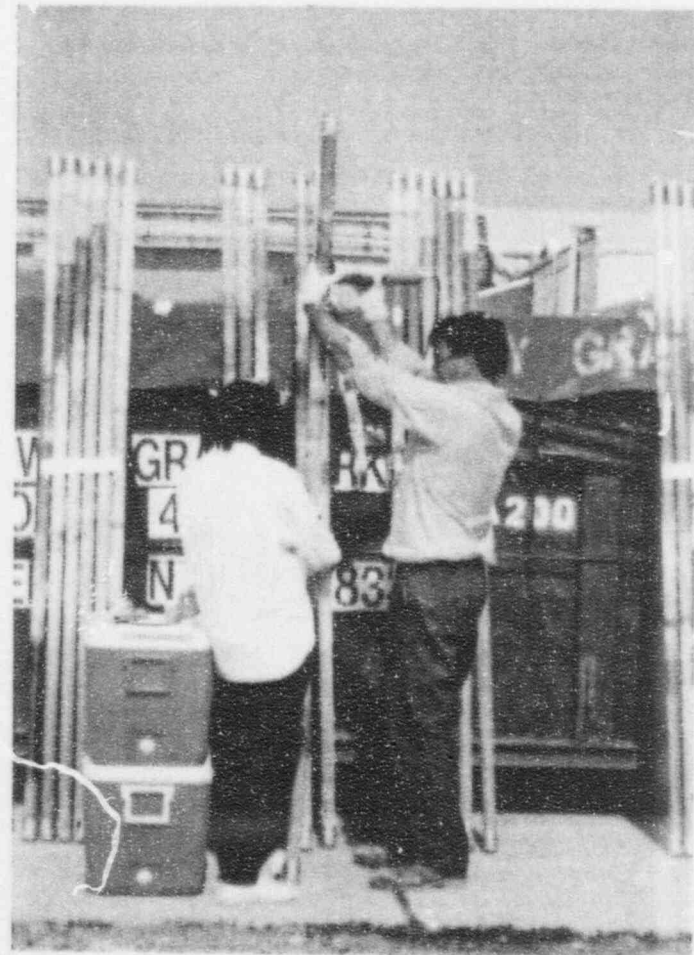
Photo 9 Spiral Survey Pattern for Field Screening The team member on the left steadily rotated the core and the team member on the right scanned along the segment downward in a constant speed ( \approx 2.5 - 4.5 cm/sec).
